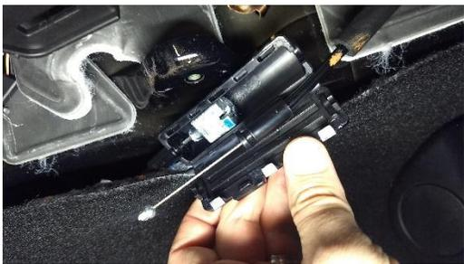
Reattach MPR cable and OEM harnesses for the USB and cup holder.
