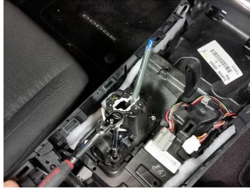
Unbolt shifter assembly from center console using 10mm socket and ratchet.
