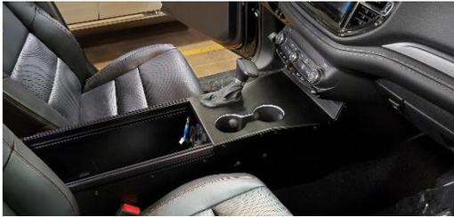
Fully tighten all hardware Run wiring as needed. Mount face plates and accessories into console with # 8 x 3/8" Torx head screws. Screws supplied with equipment
