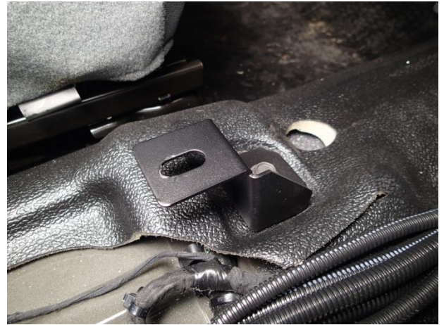
Optional CM006056 driver side forward bracket with GSM33745 (M8 x 35mm bolt) and GSM31007 (3/8 flat washer) (included in C-B66 kit)
