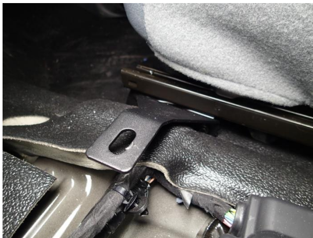
Optional CM006058 passenger side forward bracket with GSM33195 (10/32 x 3/4 screws) and GSM31003 (#10 flat washers) (included in C-B66 kit)
