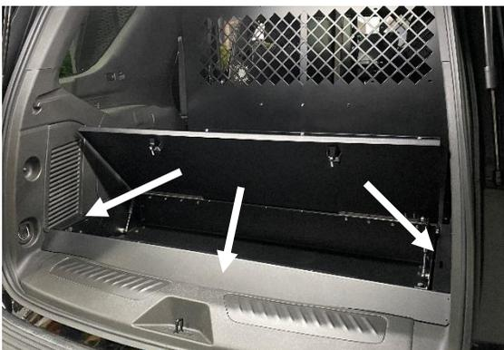
Attach rear tailgate sill trim plate to studs on box with 1/4" serrated nuts. Attach side trim with 1/4 x 3/4" hex bolts and star washers.
