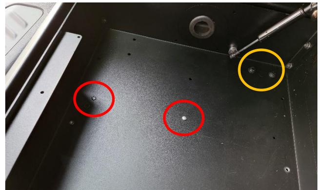
Place box into vehicle and loosely attach to floor brackets with 1/4 x 3/4" hex bolts and star washers.
