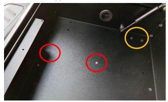
Place box into vehicle and loosely attach to floor brackets with 1/4 x 3/4" hex bolts and star washers. **Note:** After rear and side trim parts are attached. (See next step), **carefully** drill and attach tray bottom to ribs in floor with #10 x 1/2 sheet metal screws.
