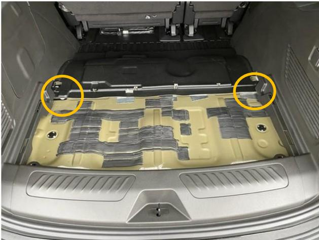
Remove OEM rear floor cover and locate existing threaded floor mount locations.
