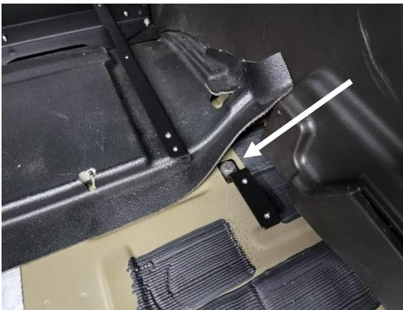
Loosely attach storage box floor bracket to OEM threaded hole with supplied M10 x 45mm bolt.
