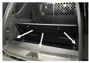
Attach rear tailgate sill trim plate to studs on box with 1/4" serrated nuts. Attach side trim with 1/4 x 3/4" hex bolts and star washers. Drill and attach screws as **noted** in previous step.
