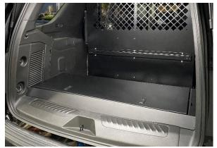
Tighten mount bracket hardware and install equipment into box as desired. C-SBX-TAH-101 Installation complete. C-TTP-TAH-101\_INST\_2-22
