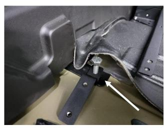
Remove OEM bolt on driver side and loosely attach storage box floor bracket to OEM threaded hole with supplied M10 x 45mm bolt.
