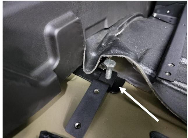
Remove OEM bolt on driver side and loosely attach storage box floor bracket to OEM threaded hole with supplied M10 x 45mm bolt.
