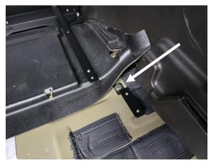
Loosely attach storage box floor bracket to OEM threaded hole with supplied M10 x 45mm bolt. Passenger side bracket shown. **Note:** Threaded hole is under foil tape.
