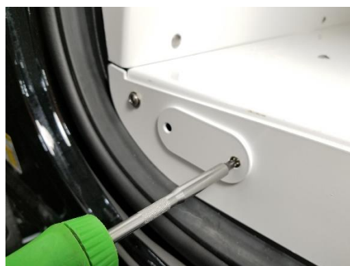
Attach 23177 cover over pass through hole in side filler panel with #10 x 1/2" flat head sheet metals screws.
