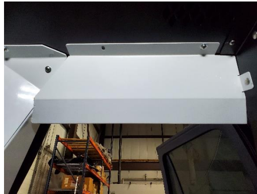
Attach upper ceiling trim panel to ceiling using (2) 1/4" x 3/4" Phillips bolts and washers.
