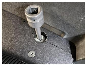
Loosely attach rear floor brackets to rear seat belt anchors on each side with OEM 12mm Torx bolts.
