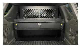
Attach riser brackets to base plate using 5/16" x 1" bolts and washers. Attach backing plate with 1/4" x 3/4" & 1/4" x 1/2" bolts and washers. Attach SBX-1000 series drawer to risers with 5/16" x 3/4" Thread-Forming Screws.
