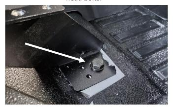
**NOTE:** Remove padding if necessary to allow supplied M10 bolt to pass through to OEM threaded hole. Repeat for both sides. Front brackets can sit on the padding.
