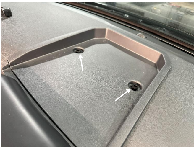
Remove OEM fasteners from upper dash pocket. Place plastic spacers over openings. (7mm socket)
