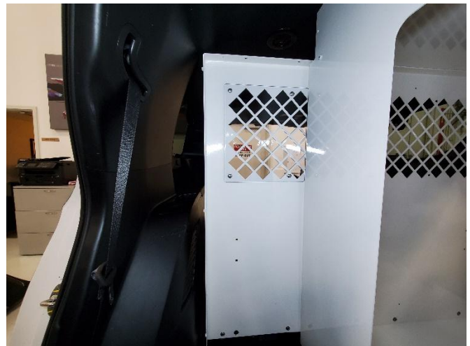
Attach divider to rear bulkhead using 1/4" x 3/4" Phillips bolts and flat washers.
