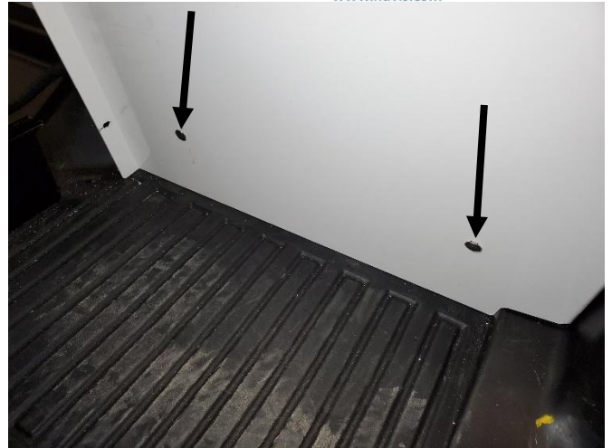
Attach bulkhead to floor mount bracket using 1/4" x 3/4" carriage bolts and serrated nuts.
