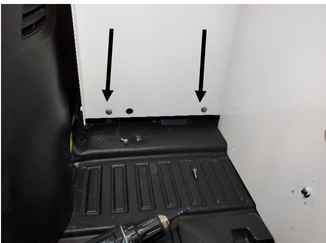
Be sure to attach passenger side of lower rear bulkhead to rear cargo filler plate using 1/4" x 3/4" Phillips bolts and flat washers.
