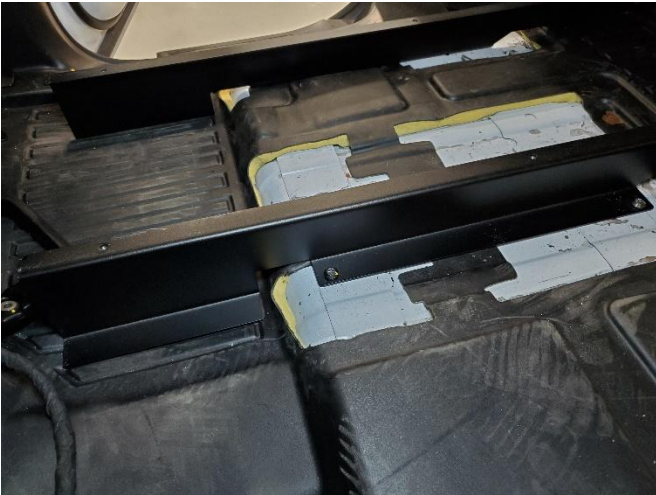
Repeat for middle bracket. Do not tighten hardware yet.
