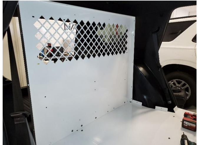
Install rear bulkhead using 1/4" x 3/4" Phillips head bolts and flat washers.
