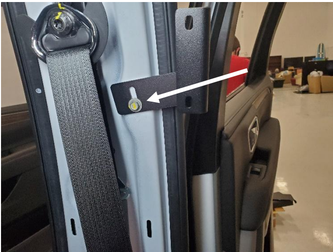
Remove passenger side grab handle and upper trim panel from B pillar. Attach upper mounting bracket using OEM hardware and reinstall panel.
