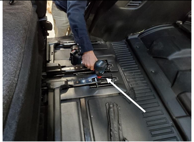
Flip seat seats forward to access hardware.
