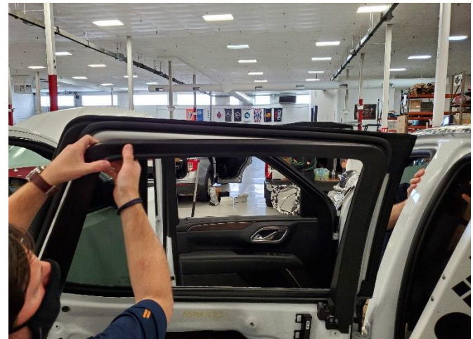
Gently remove trim around window frame.
