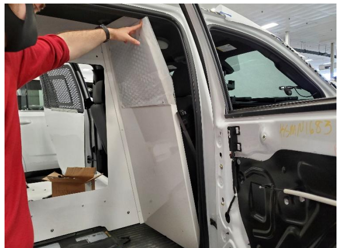
Place passenger front bulkhead into vehicle and attach to divider wall using 1/4" x 3/4" carriage bolts and serrated nuts.
