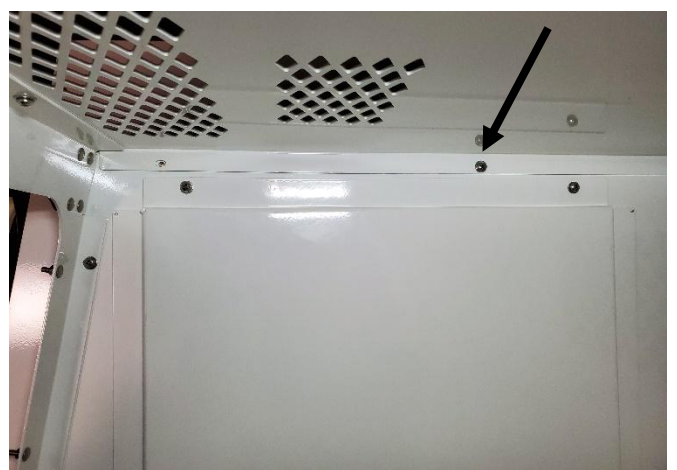
Attach ceiling to front middle divider using 1/4" x 3/4" Phillips head bolts and flat washers.
