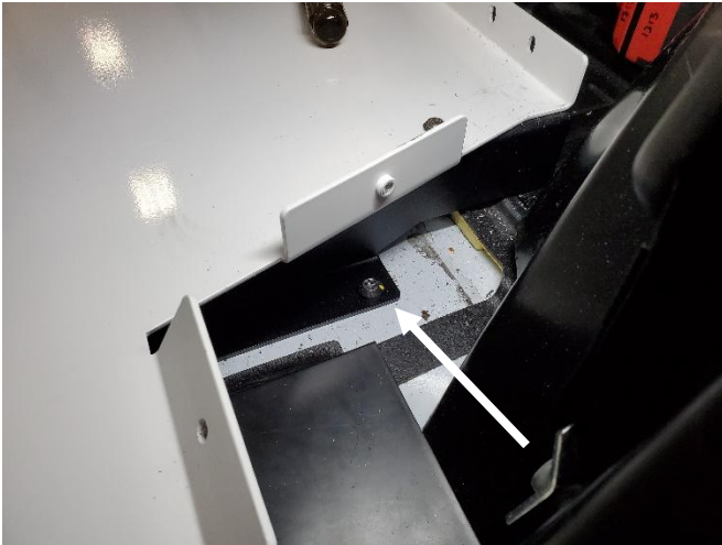
Tighten rear floor mounting hardware.
