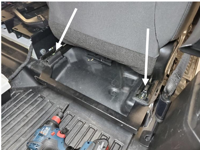
Remove rear seat bolts from front passenger seat. Place lower prisoner side bulkhead floor mount bracket under seat rails. Attach bracket and seat rails reusing OEM hardware.
