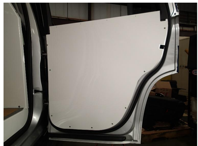
Hook top of door panel into rubber window gasket. Center door panel and drill 1/8" mount holes. Attach with # 10 x 3/4" sheet metal screws.
