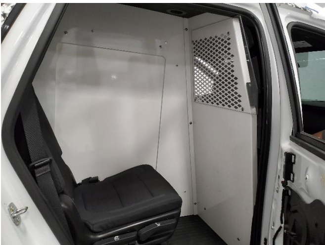
Re-install previously removed OEM seat.
