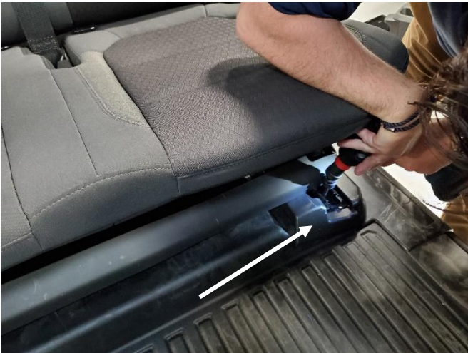
Flip seat seats down and remove plastic trim covers to access front hardware.
