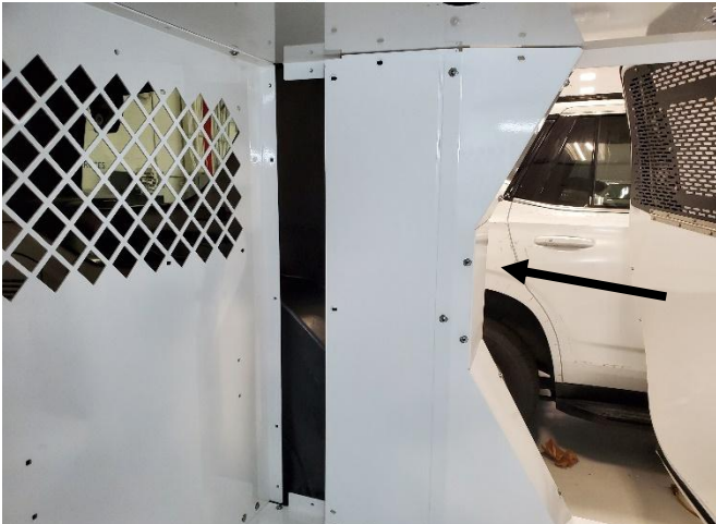
Sub-assembly K9 inner side filler, outer side filler, and filler extension panels outside of insert using 1/4" x 3/4" Phillips head bolts and flat washers.
