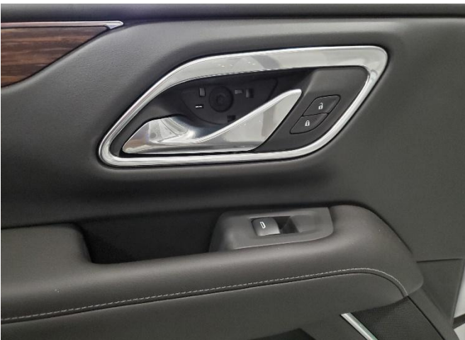
Remove plastic covers behind the paddle handle. Remove screws. (7mm socket)
