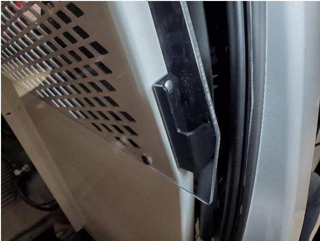
Attach bulkhead to B pillar bracket using 1/4" x 3/4" carriage bolts and serrated nuts.
