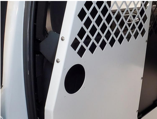
Place K9 bulkhead into vehicle and attach to B pillar bracket using 1/4" x 3/4" carriage bolts and serrated nuts.
