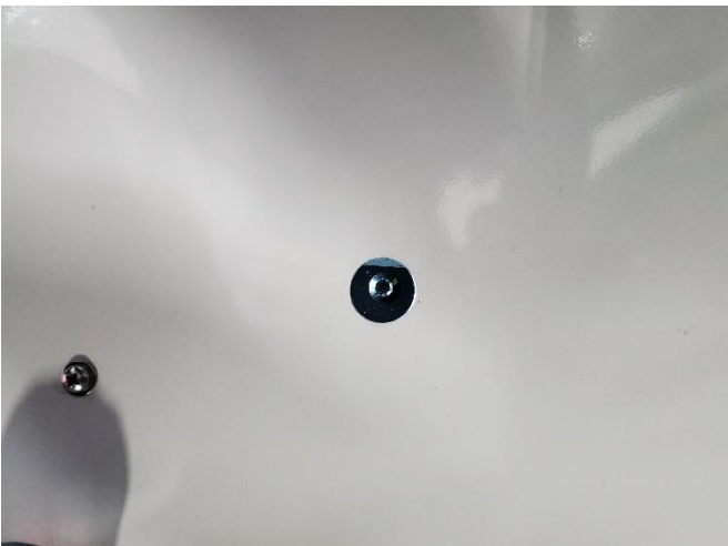
After floor hardware has been attached, tighten OEM mounting hardware through holes in floor.
