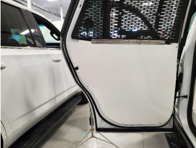
Align window guard hinge mounting holes to holes in the door panel. Attach hinge with # 10 x 1/2 Phillips pan head sheet metal screws.
