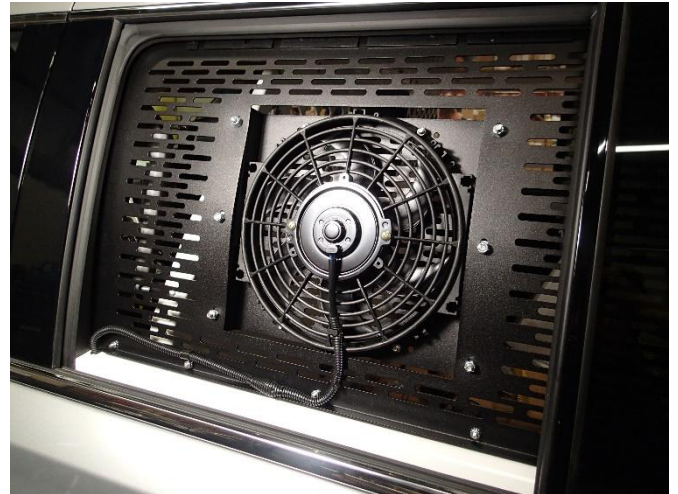
Mount optional K9-A-104 Fan and Fan mount to window guard with 1/4" hardware and spacers as per the instructions provided in the K9-A-104 kit.
