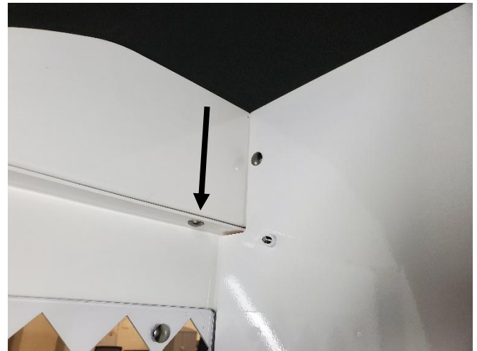
Place rear passenger side top trim panel onto rear bulkhead and attach using 1/4" x 3/4" carriage bolts and serrated nuts.
