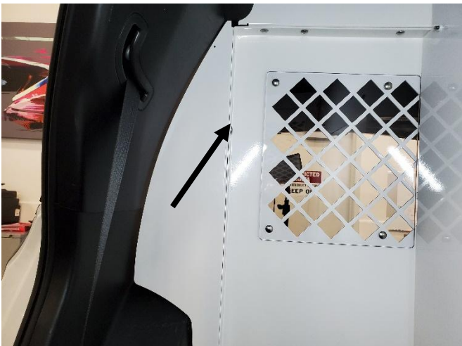
Install rear passenger side trim panel onto rear bulkhead and attach using 1/4" x 3/4" carriage bolts and serrated nuts.
