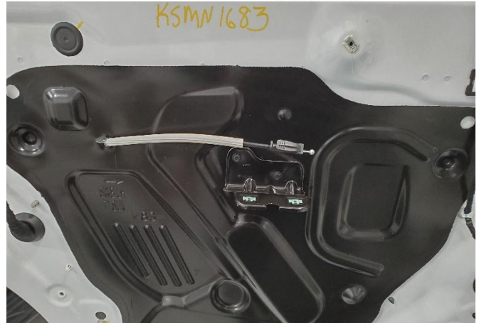
Remove / unsnap entire door panel from door. Remove armrest bracket. (7mm socket)
