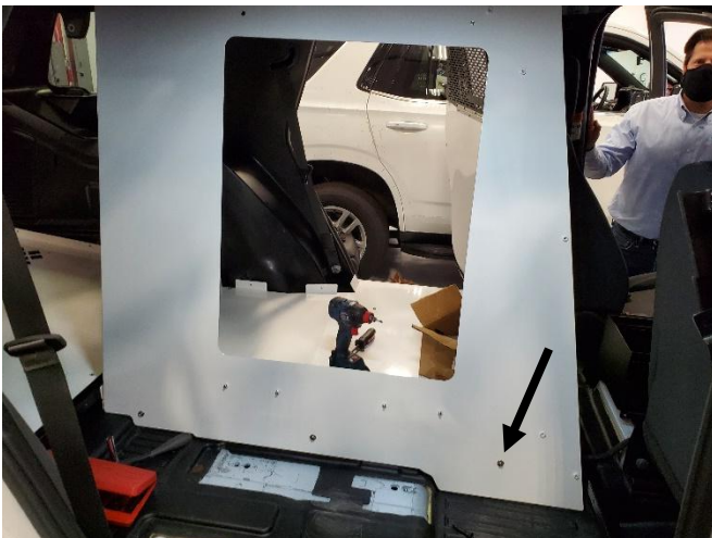
Install divider wall into vehicle and attach to floor using 1/4" x 3/4" Phillips bolts and flat washers.
