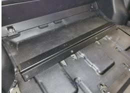
Attach the middle floor, mounting bracket using supplied M10 x 70mm bolts and 7/16" flat washers.
