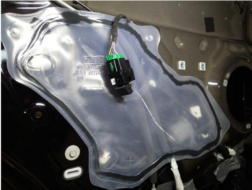
Remove the window switch from the door and relocate the harness. The switch should be placed between the moisture barrier and K9 door panel.
