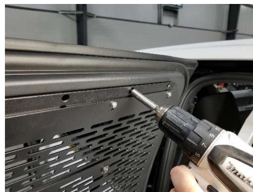
Attach upper window bracket to door frame using #10 x 1/2" flat head screws.
