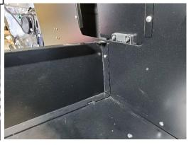
Attach to lower front bulkhead using 1/4" x 3/4" Phillips head bolt and washer.
