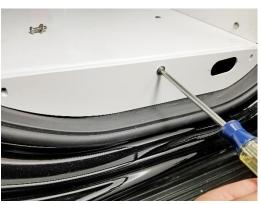
Attach lower side filler trim panels using 1/4" x 3/4" Phillips head bolts and washers.
