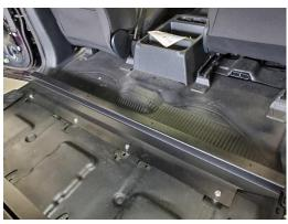
Place the .77" spacers at the front and attach front bracket using (4) previously removed OEM seat bolts.
