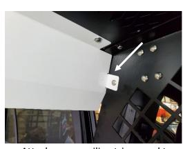
Attach upper ceiling trim panel to front bulkhead using carriage bolt and serrated nut.
