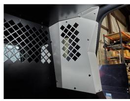
Attach upper side trim panel to rear wall lower corner trim panel and upper forward side trim panel using 1/4" x 3/4" Phillips bolts and washers.
