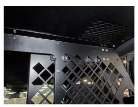
Attach front using 1/4" x 3/4" Phillips head bolts and washers.
