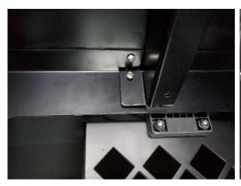
Attach to upper front bulkhead using 1/4" x 3/4" Phillips head bolt and washer.
