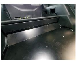
Attach rear floor section to forward floor section and rear floor, mounting bracket using 1/4" x 3/4" Phillips bolts, and washers.
