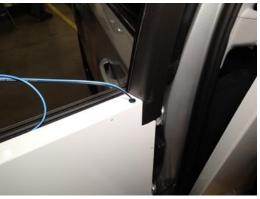
Place K9 door panel onto the door. Be sure to route the wires for the optional K9-A-104 window fan at this time.
