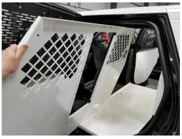
Place front bulkhead floor into vehicle and attach using 1/4" x 3/4" carriage bolts and serrated nuts.
