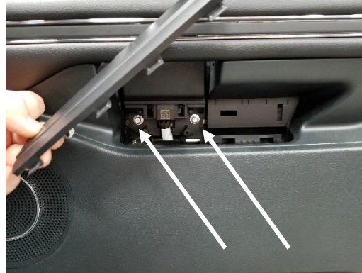
Remove two (2) bolts behind access cover in middle of door panel. (8mm socket)
