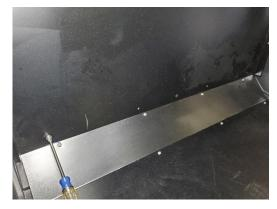
Attach rear bulkhead to floor using 1/4" x 1/2" Phillips head bolts and washers.
