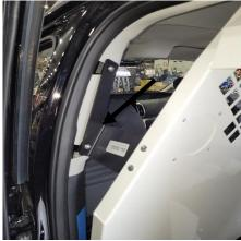
Attach upper mounting brackets using 1/4" x 3/4" Phillips bolt and washer.
