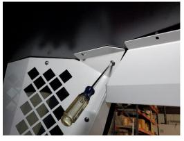
Attach upper ceiling trim panel to upper side trim panel using 1/4" x 3/4" Phillips bolt and washer.
