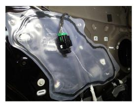
Remove the window switch from the door and relocate the harness. The switch should be place between the moisture barrier and K9 door panel.
