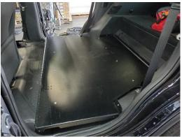
Place floor in vehicle and loosely attach using 1/4" x 3/4" carriage bolts and serrated nuts on the front bracket, 1/4" x 3/4" Phillips bolts, and washers on the back bracket.
