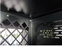
If using optional K9-A-112 divider, place in kit at this time. Attach to rear wall using (2) 1/4" x 3/4" Phillips head bolts and washers.
