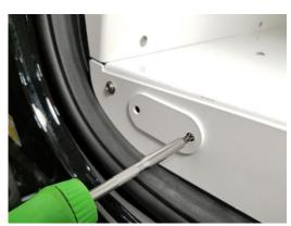
Attach 23177 cover over pass through hole in side filler panel with #10 x ½"flat head sheet metals screws.
