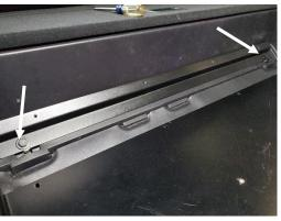
Install rear floor, mounting bracket using OEM hardware.
