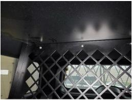
Place ceiling in kit with the lip hanging over the rear bulkhead. Attach using 1/4" x 3/4" Phillips head bolts and washers.
