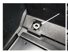
Remove rear covers and hardware from forward side, corners of cargo area storage pocket. Install 1" spacer, repeat for other side.
