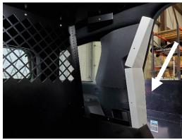
Attach upper, forward side trim panel to lower corner trim panel using 1/4" x 3/4" Phillips bolt and washer.
