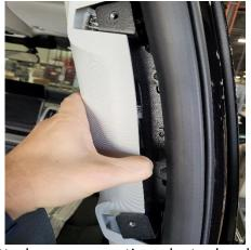
Attach upper mounting adapter brackets using previously removed OEM hardware.
