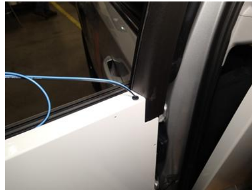
Place K9 door panel onto the door. Be sure to route the wires for the optional K9-A-104 window fan at this time.
