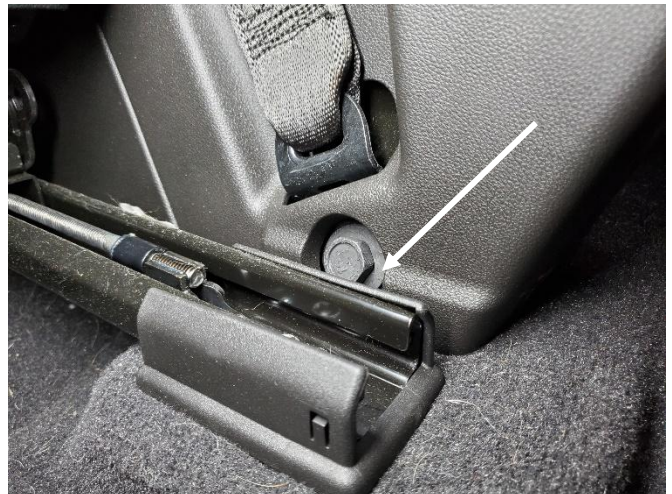
The rear bolts are obstructed by the seat rail.
