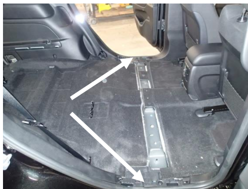
Remove lower side step sill trim. Save trim to be modified and reused. (Trim panel removal tool)
