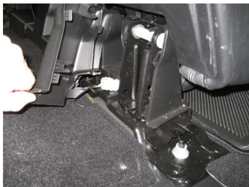
Remove plastic covers as needed to access seat bolts. Remove seat hardware and save. (15mm socket)
