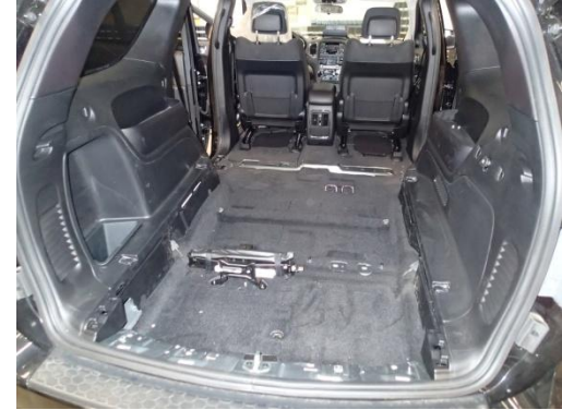
Remove rear cargo floor and storage compartment. (10mm socket and Phillips screwdriver)
