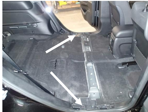
Remove lower side step sill trim. Save trim to be modified and reused. (Trim panel removal tool)
