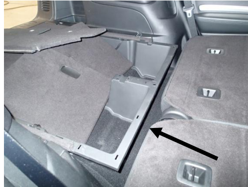
Unsnap and remove cargo floor extension / cover panel.
