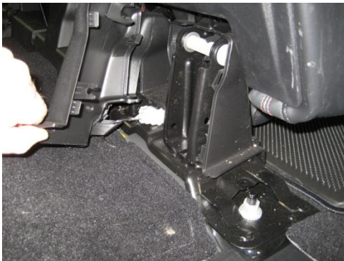
Remove plastic covers as needed to access seat bolts. Remove seat hardware and save. (15mm socket)
