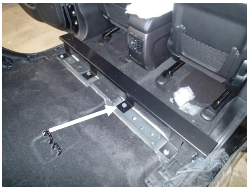
Use OEM nuts and bolts to attach forward K9 kit floor bracket to seat mount locations.
