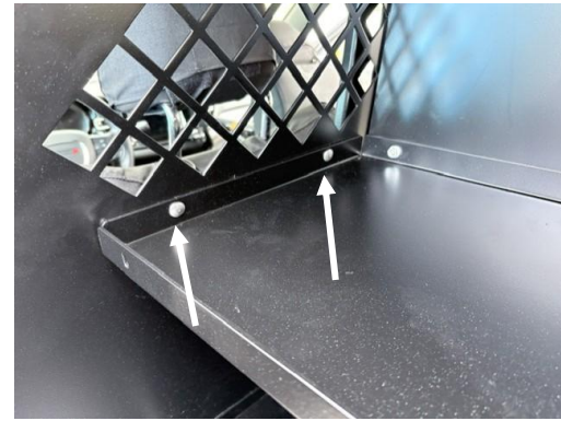
Loosely attach top shelf to front bulkhead using two (2) 1/4" x 1/2" carriage bolts and serrated nuts.
