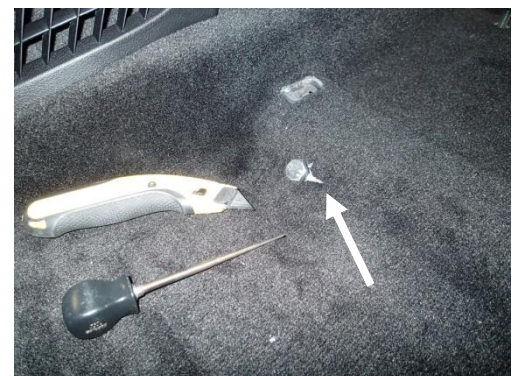
Using a scribe and razor knife, locate the rear mounting holes and cut carpet at hole location as shown.
