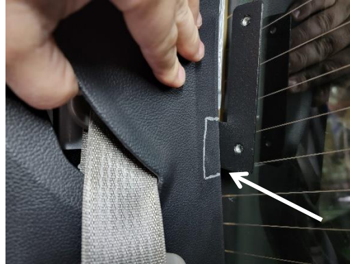
Mark section of trim to be notched to allow clearance for bracket.
