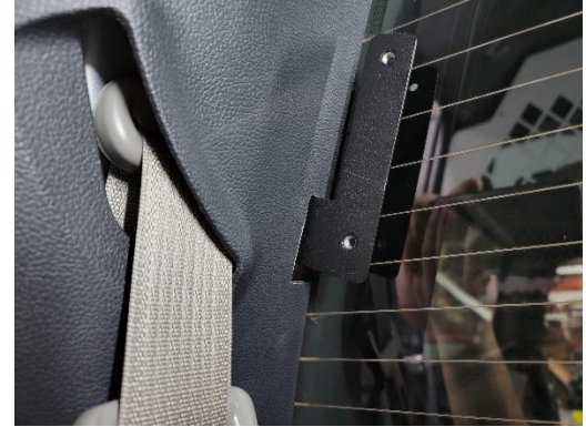
Snap trim back into place once clearance notch has been cut.
