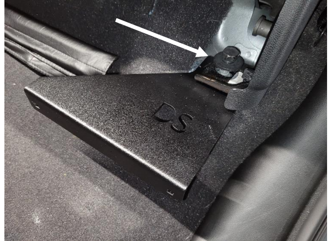
Loosely attach driver side bracket to OEM driver side rear seat floor bolt.
