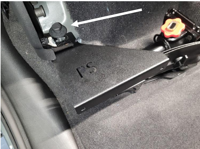
Loosely attach passenger side bracket to OEM passenger side rear seat floor bolt.
