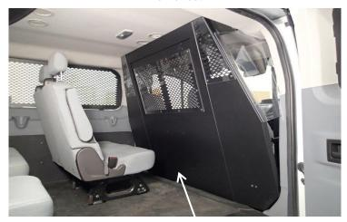
Slide partition in through the side door and prop into position. Attach to the front lower support brackets using two (2) 1/4"x 3/4" carriage bolts and 1/4" nuts.
