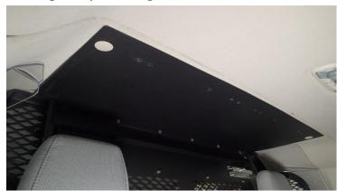
Remove push pins from headliner and line up mounting plate to the holes. Reinstall push pins to align the plate to the rib. Pre-drill 1/8" holes and install with #10 x 1-1/4" flat head sheet metal screws.
