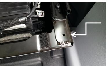
Slide front passenger seat forward and remove cover under seat. Drill out the existing outboard hole in seat base to 1/4".
