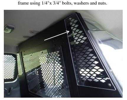
Install additional clear polycarbonate wings using 1/4"x 3/4" carriage bolts, washers, and nylock nuts.
