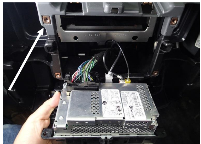
Remove radio mount screws, unplug and remove radio control. (7mm socket)
