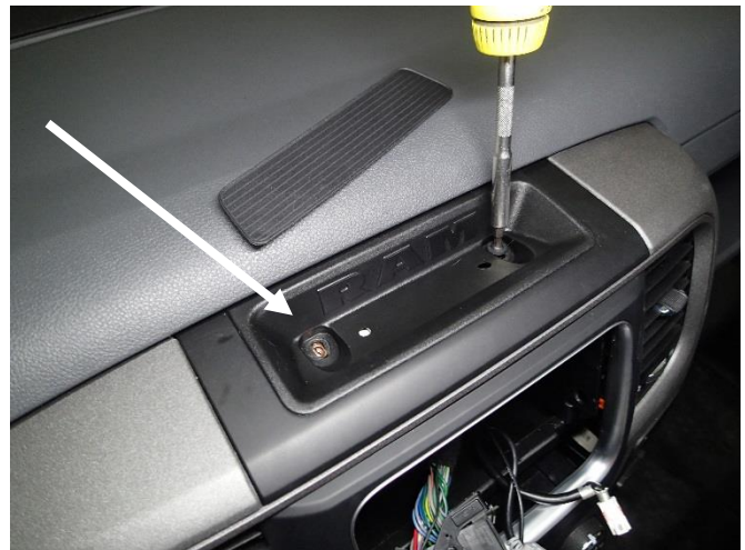
Remove rubber liner and remove screws in upper center coin tray. (T20 Torx bit)
