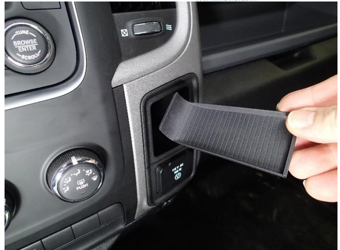
Remove rubber liner in lower right dash pocket.
