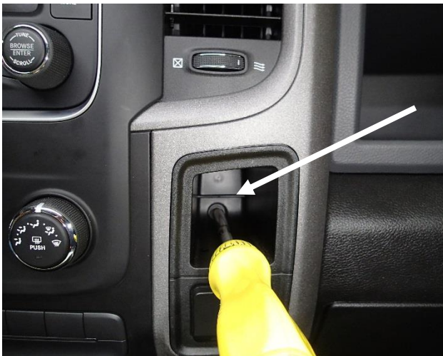
Remove screw in lower right dash pocket. (T20 Torx bit)
