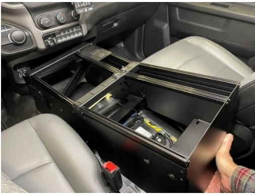
Carefully place console housing into vehicle on top of OEM center seat brackets.
