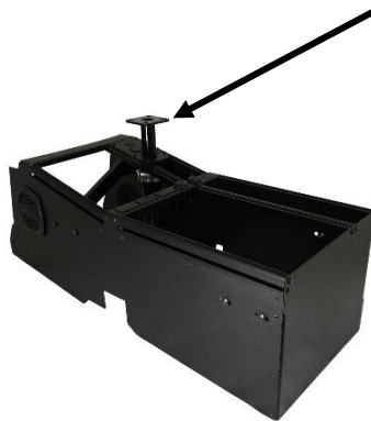
Optional C-HDM-214 pole can be installed at this time using the existing 1/4" x 3/4" carriage bolts in the side of console. Remove round knockout in pole face plate and attach plate to console around pole.
