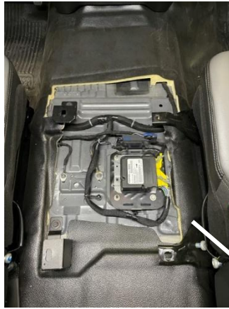
Remove center seat and front accessory pocket. Leave OEM center seat brackets in vehicle.
