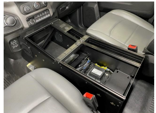
Console housing installed and ready to complete wiring, control head, and accessory installation. Slide 1/4-20 hex nuts (provided) into side extrusions as needed for side mounted accessories
