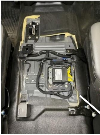
Remove center seat and front and floor shift rod with knob. Leave OEM center seat brackets in vehicle.
