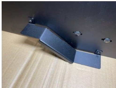
Attach cover plate on passenger side of console with supplied Torx screws. This can be done after console is installed, but passenger seat would need to be removed for access.
