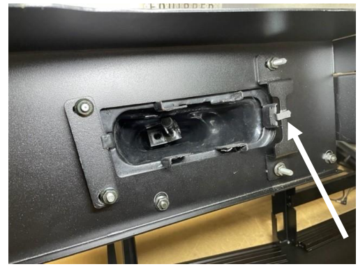
Attach rear shifter boot retaining / adaptor plate (27215) on rear studs with 1/4-20 serrated nuts. Clip on rubber boot onto plate.
