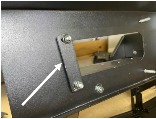
Place front shifter boot retaining / adaptor plate (27275) on spacers and attach with 1/4-20 serrated nuts.
