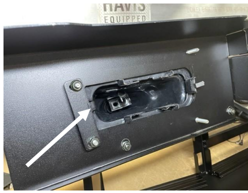
Place OEM shifter with rubber boot into cutout and clip onto front retaining plate.
