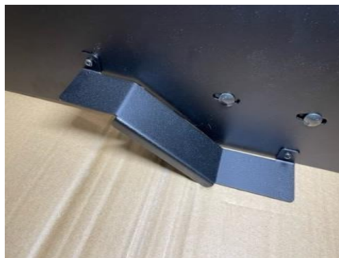
Attach cover plate on passenger side of console with supplied Torx screws. This can be done after console is installed, but passenger seat would need to be removed for access.
