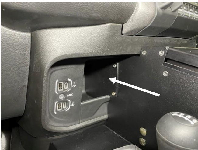
Attach driver side forward trim panel with supplied Torx screws.
