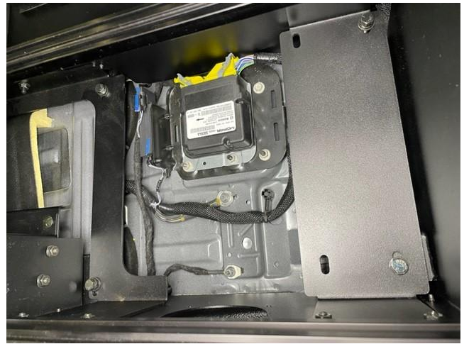
Attach console floor brackets to OEM seat brackets with 5/16-18 X 3/4" Hex bolts, flat washers, lock washers and nuts.
