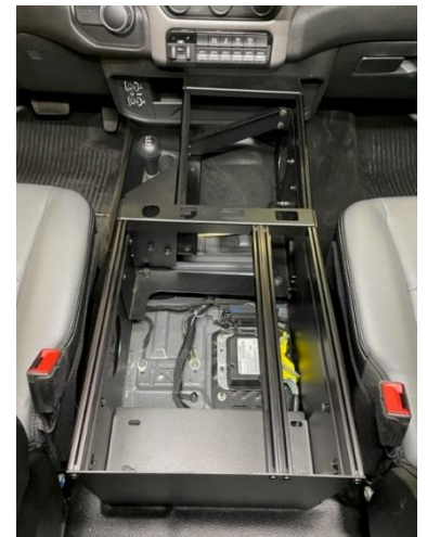
Carefully place console housing into vehicle on top of OEM center seat brackets.
