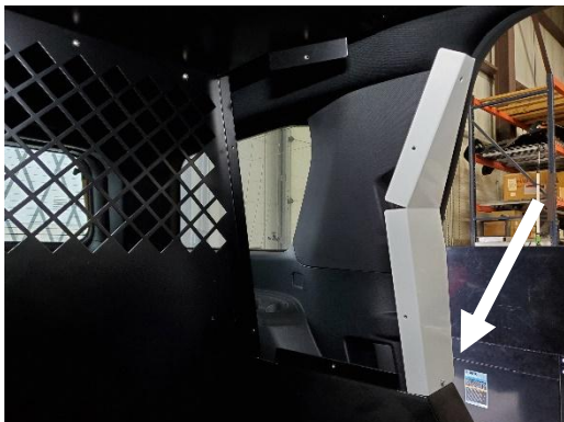
Attach upper, forward side trim panel to lower corner trim panel using 1/4" x 3/4" Phillips bolt and washer.
