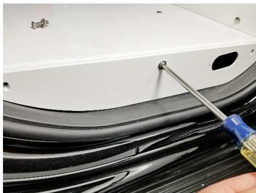
Attach lower side filler trim panels using 1/4" x 3/4" Phillips head bolts and washers.
