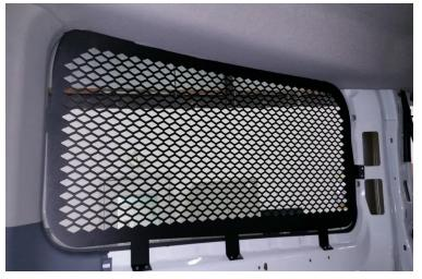
Hang the screen with only a few screws and then mark and drill the remaining mounting holes.
