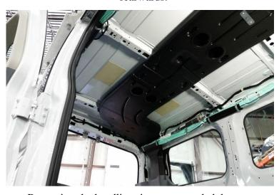
Removing the headliner is recommended, but not required. Removing the headliner will be required if installing a Middle Partition.
