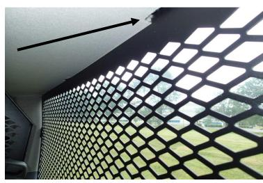
The headliner will need to notch around the tabs so that it sits properly above the screens.
