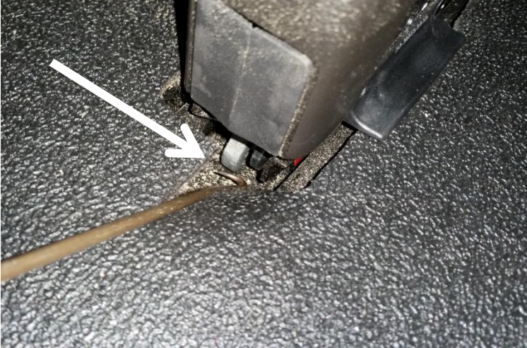
Remove the rear seats out of the van. Start by grabbing the seat release with a long hook style pick tool.
