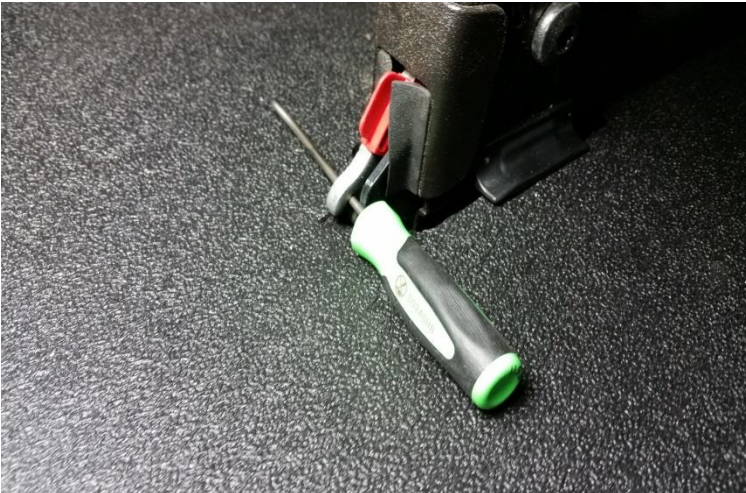
The latch will relock itself once you let go. Use another pick tool or small screwdriver to keep the latch released while you release the other side.
