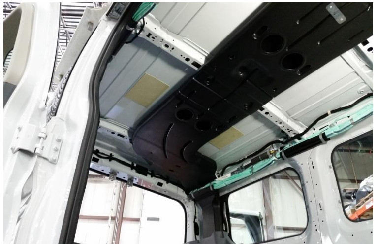
Removing the headliner is recommended, but not required. Removing the headliner will be required if installing a Middle Partition.
