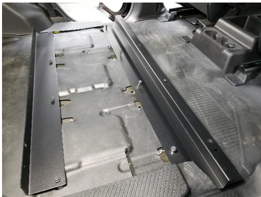
Place the .77" spacers at the front and attach front bracket using (4) previously removed OEM seat bolts.
