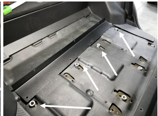
Place the larger 1.5" spacer over the (4) rear bolt holes corresponding to the rear floor mounting bracket.
