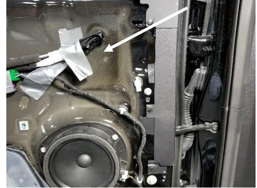
Tape the lock rod and door handle release cables along the upper alcove of the door to keep them clear.
