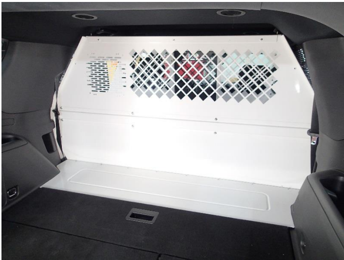
Confirm smooth functionality of the rear storage cover. Cover is designed to rest under the lid of the OEM forward storage compartment.
