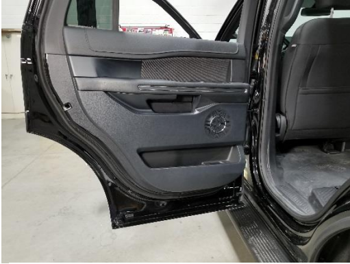
Remove rear passenger door panels first.
