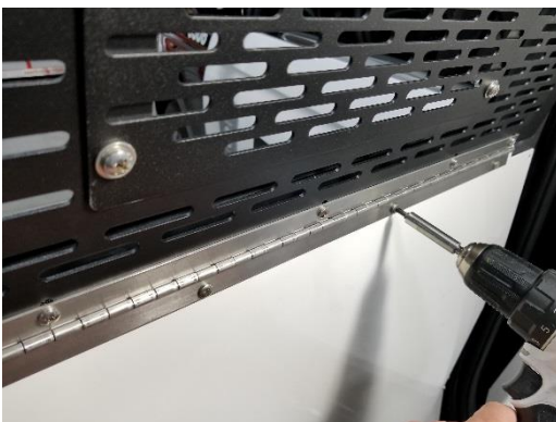
Attach window screen to door panel using #10 x 1/2" screws.
