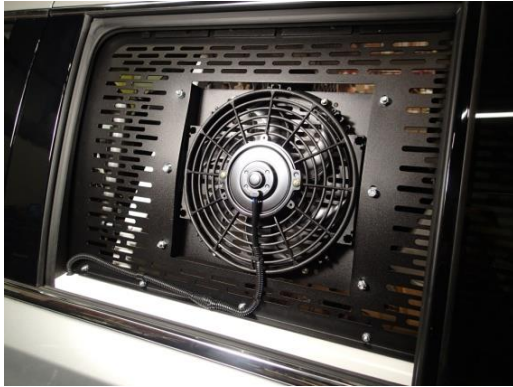
Wire fan with previously run wires and secure harness.
