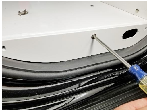
Attach lower side filler trim panels using 1/4" x 3/4" Phillips head bolts and washers. (Floor parts are black)
