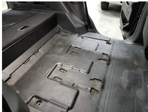
Remove the rear seats from the vehicle. Set hardware aside for later use.
