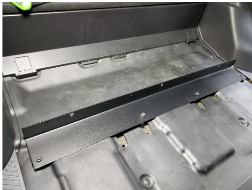
Attach the rear floor mounting bracket using supplied M10 x 70mm bolts and 7/16" flat washers.
