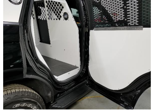
Once caulk is dry. Place the rubber mat in kit.
