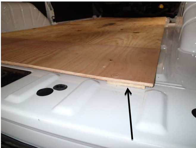
Overall length of plywood should be at least 102" long (for 100" insert) or 122" long (for 120" insert) to match insert length plus rear sill trim. Additional piece needed for side entry area. Cut 4x4" square spacers and install in corners as shown. These prevent the wood from bowing when the kit is bolted down later.
