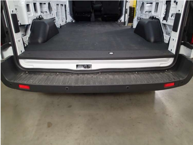
Remove factory rubber mat and rear floor trim.
