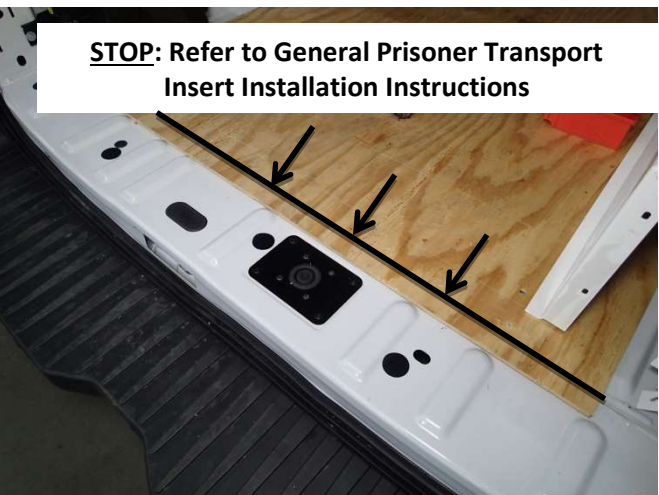
See General Prisoner Transport Insert Installation Instructions and loosely fit parts before installing any trim or bolting parts to floor.
