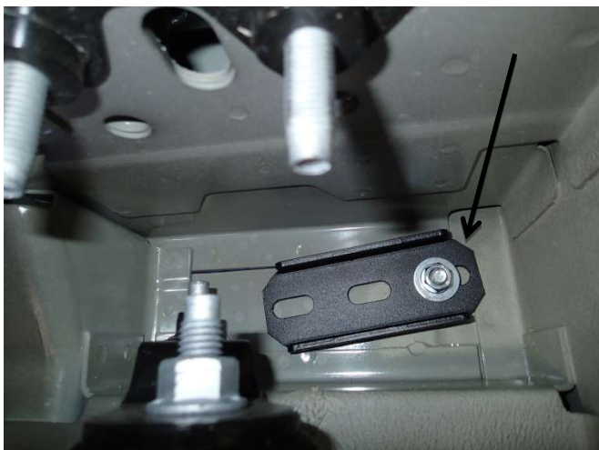
Be sure to use the fender washer when installing the lock washer and nut.
