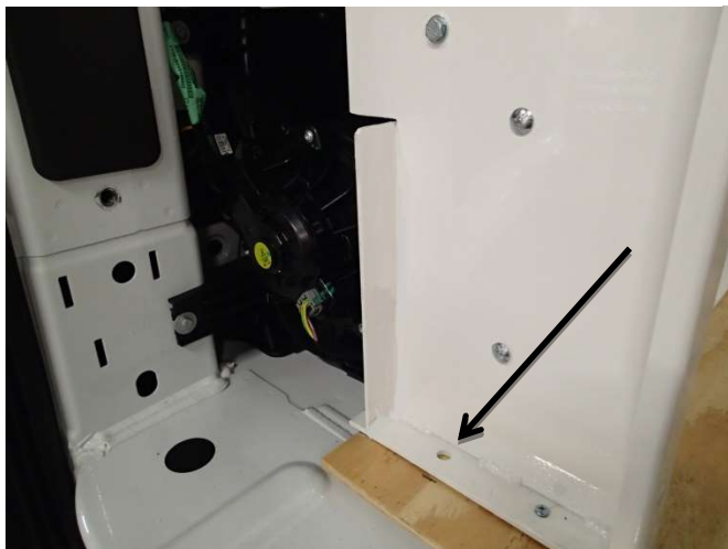
Use the outer mounting hole on the rear door frame on the single compartment. This will allow the bolt to drop between two frame supports.
