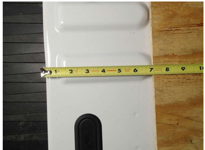
Space plywood 7" forward from rear center of van.
