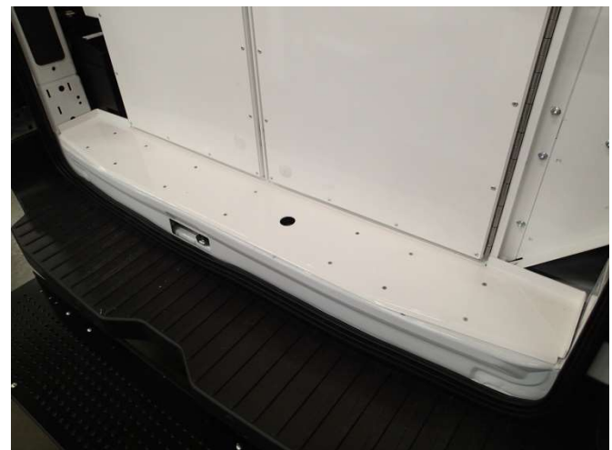
Line up rear door sill (KKM006910) to the rear bulkhead. Spare tire access hole should be centered over release. Install fourteen (14) #10 screws through pre-punched holes in sill plate. Do not over tighten screws.
