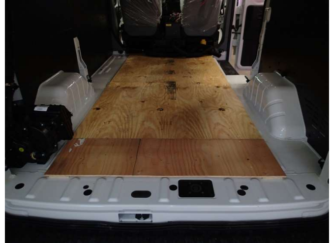
Cut and install 1/2" thick plywood subfloor Approximately (2) 1/2 x 48" x 96" sheets required. (Plywood and flat head screws not included with kit)
