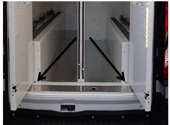
On the double and triple compartments you will use the holes on the outer portion of the door frame.
