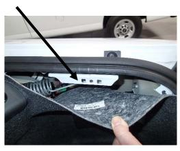
Photo shows 2019 without cargo hook and trunk liner pulled down. The existing OEM metal bracket has holes that must be avoided when mounting TSM upper bracket. Properly position TSM so upper bracket holes are outboard of OEM holes.
