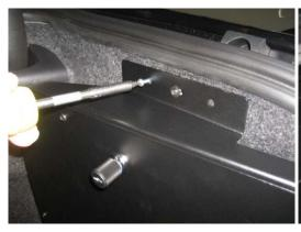
Drill 5/32"holes at upper bracket (next to OEM screw) and attach with # 10 x 3/4" Sheet metal screws
