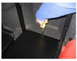
Attach lower frame to floor with # 10 x 3/4" sheet metal screws.
