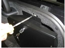
Place Trunk Side Mount frame assembly into position and attach to inner fender with previously removed Cargo hook screw into original hole.
