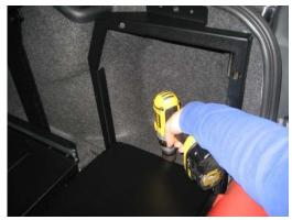
With Trunk Side Mount in position, drill three 5/32" holes into floor.
