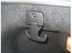
Remove side cargo hook. Mount screw to be reused later.
