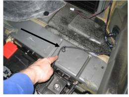
Unclip and move wiring at side floor area. Make sure it is repositioned so it will not get damaged.
