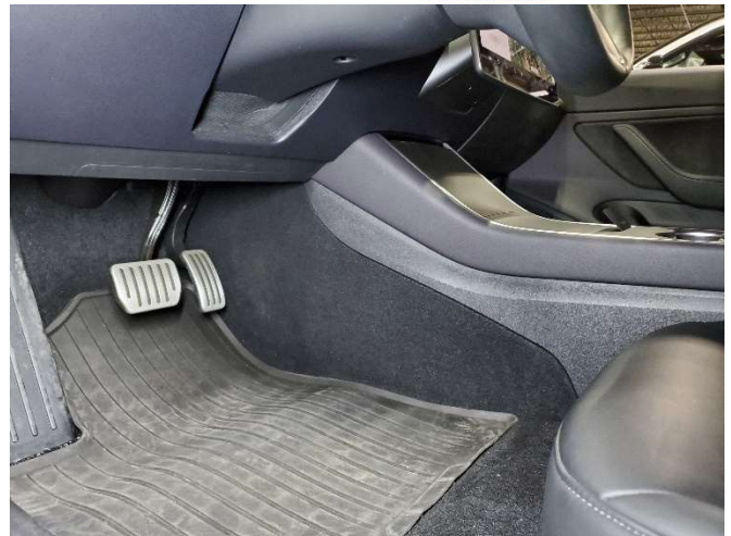
Remove carpeted side trim from side of center console.
