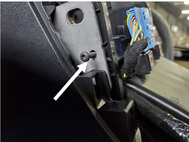
Unbolt rear cross brace from console.
