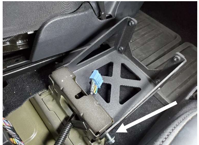
Attach rear-mounting bracket to floor using previously removed 10mm head bolts.
