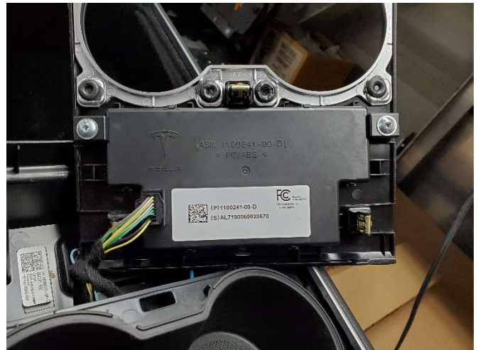
Remove proximity card sensor from console trim.
