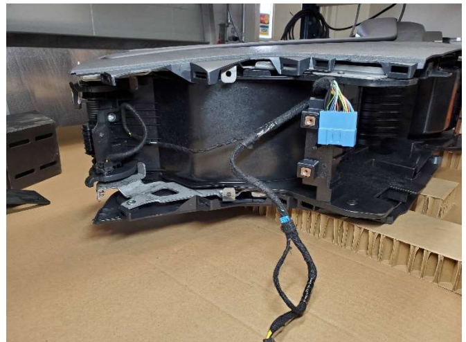
Remove harness from console.
