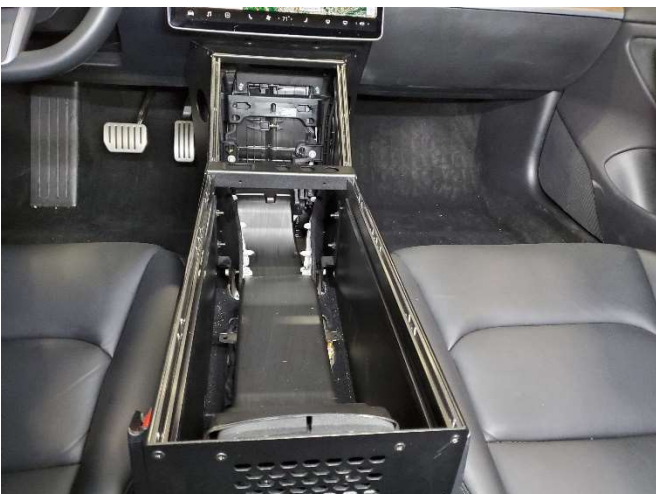
Slide Havis console into the vehicle and up against the dash.
