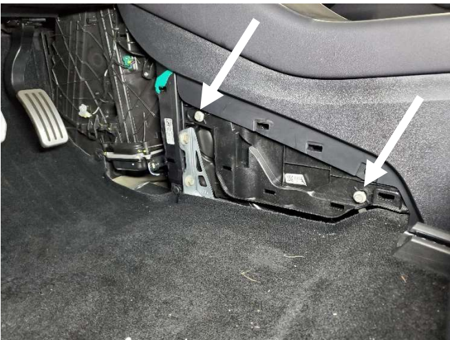
Remove (2) 10mm head bolts. (Repeat for other side)
