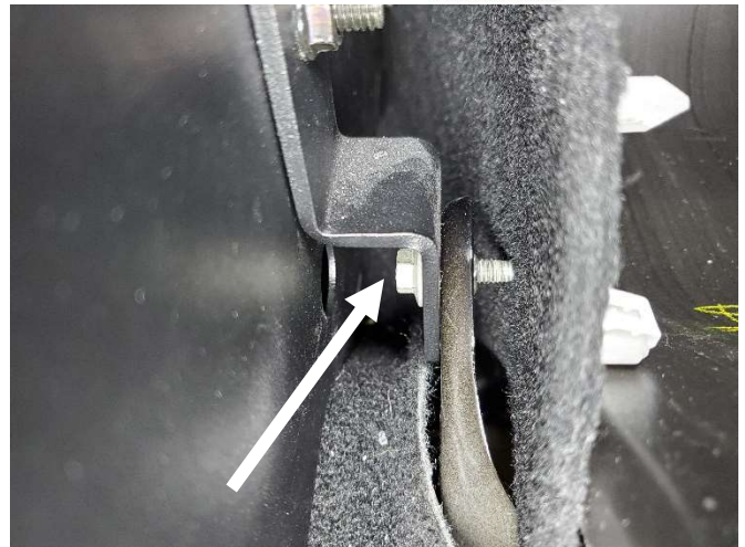
Attach OEM 10mm head bolt into bracket.
