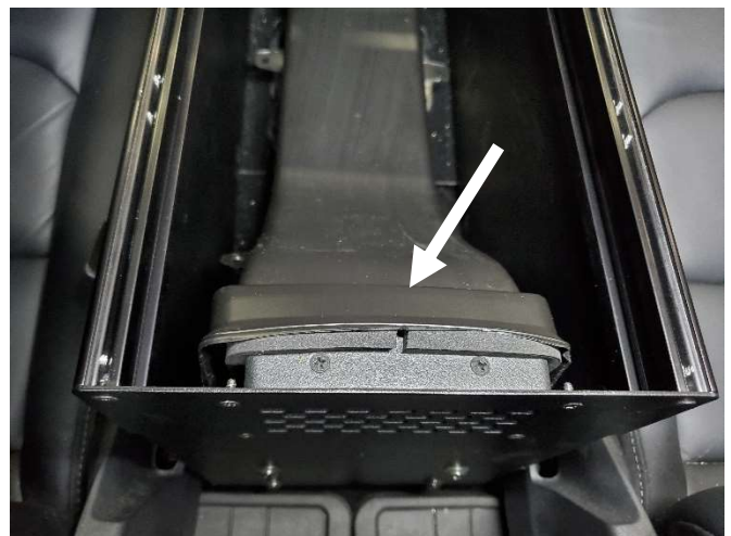
Line up ductwork to rear end of console housing. Add supplied foam strips to console prior to installing ductwork.
