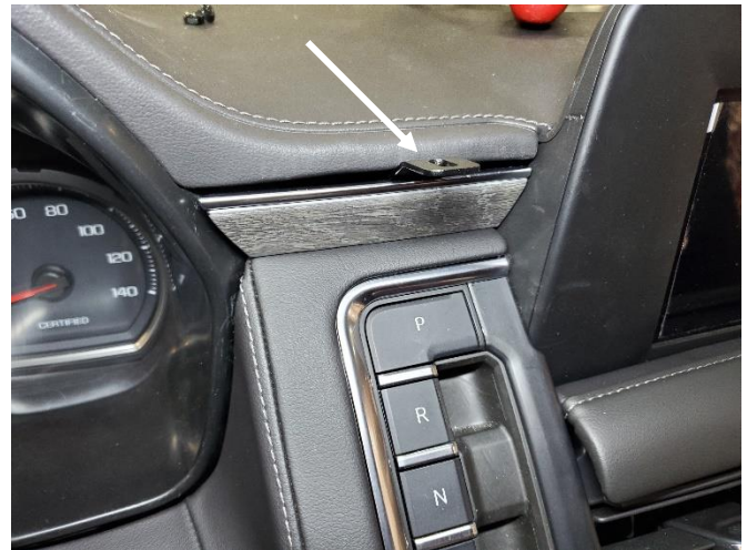
Snap back in upper driver side dash trim allowing mounting bracket to stick out the top.
