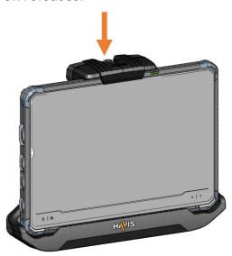
**3.** Once unlatched, remove the tablet by rocking the top of the tablet away from the docking station and carefully lift out of the docking station, top end first.
