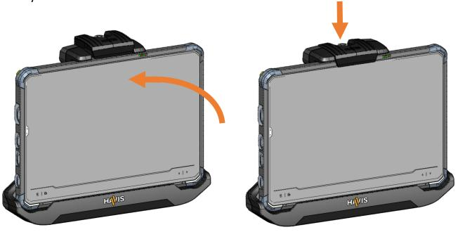
4. For theft deterrence, secure tablet by locking the docking station with the supplied key (Hardware Kit Item 2)
