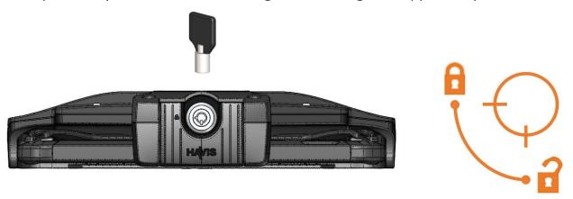
**2.** While securely holding the tablet, push the lock button on the top of the docking station until the latch hook releases.
