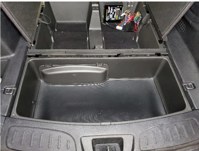
Remove rear storage cover, this unsnaps from the base.
