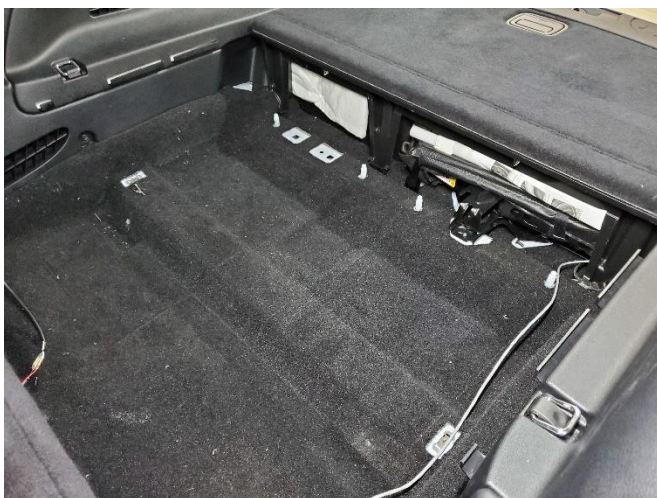
Remove forward storage pockets from vehicle. These will not be reused.
