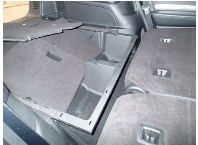
Flip down rear seats, unsnap forward storage pocket covers, and forward trim.
