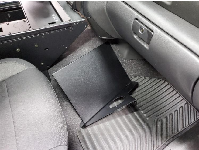
Slide equipment mounting plate in front of console. This can be installed prior to placing console in vehicle if desired.
