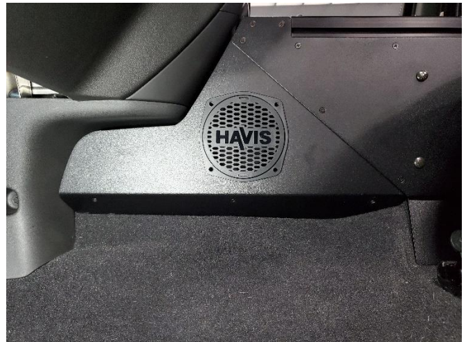
Snap speaker grills into side of console.
