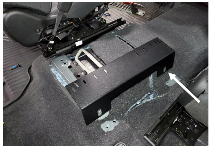
Attach floor mounting brackets using previously removed OEM hardware. Use 1/2" spacers at front between bracket and Trans hump. Seal off (plug) vent duct with block of foam provided.
