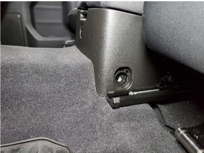
Remove OEM bolts using 18mm socket
