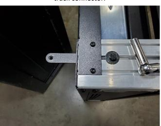
Install the 1/4" bolt, split lock washer, and flat washer.
