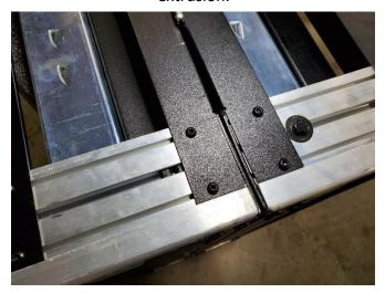
Slide additional SBX-1000 onto the track connector.
