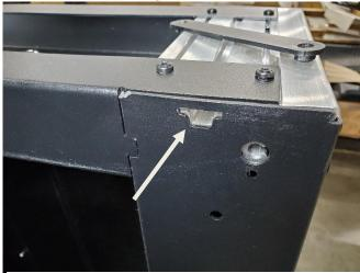
With SBX on its side, locate the slot for the track connector.
