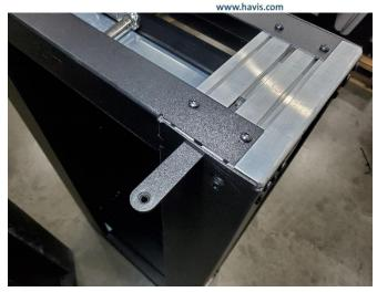
Insert track connector about halfway in to extrusion.
