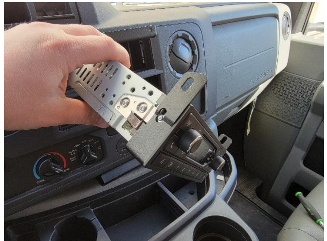
Slide up until snug on radio chassis.
