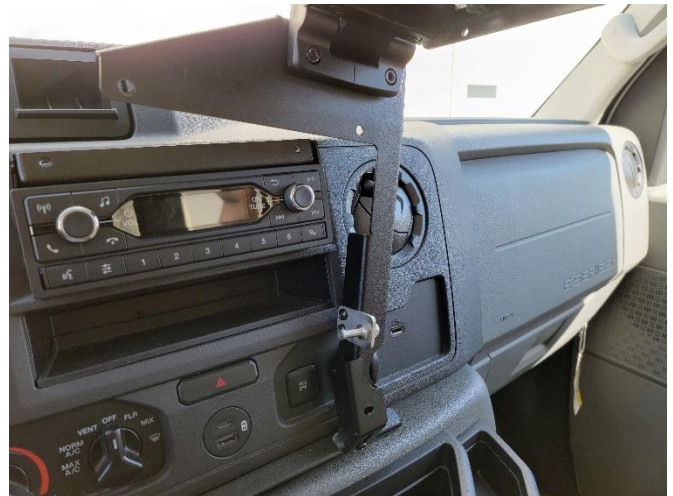
Place upper frame assembly onto lower frame.
