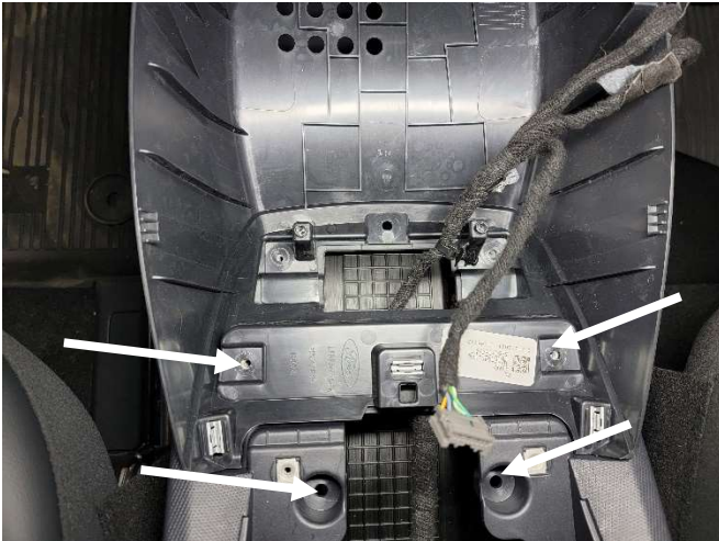
Remove (4) OEM fasteners from rear of lower, center storage area.
