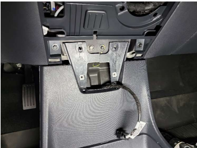
Remove lower, center storage area.
