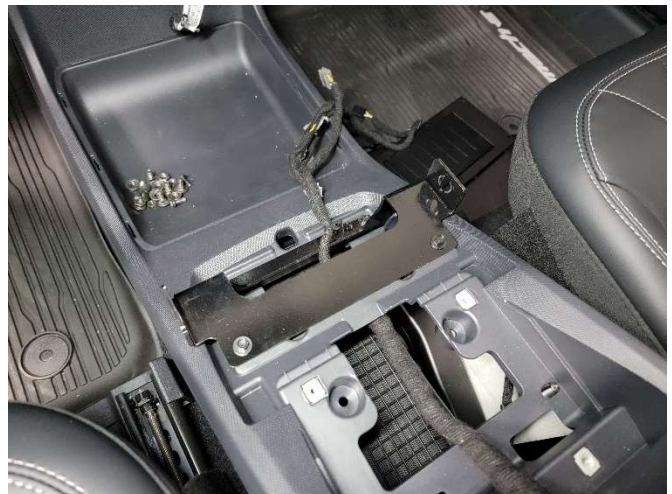
Attach the rear mounting bracket using previously removed OEM fasteners.
