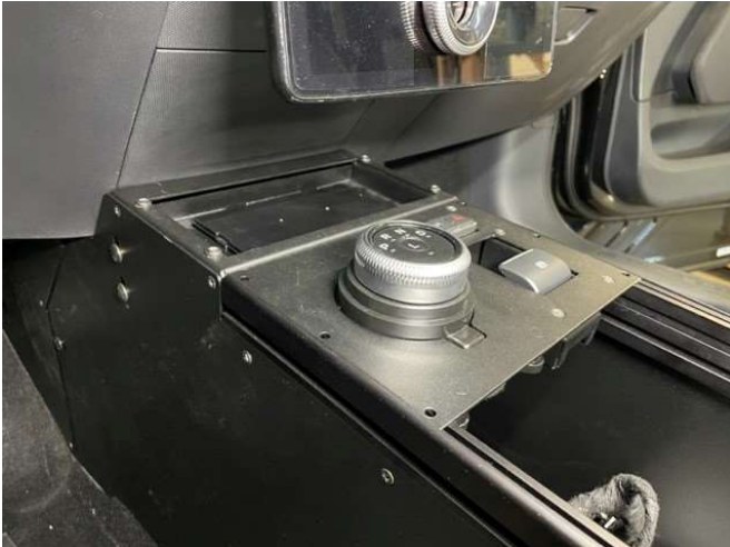
Install charger bracket and shifter plate assemblies into console.
