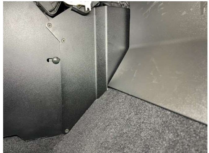
Install passenger side trim panel with three (3) #8-18 X 3/8 flat head screws.
