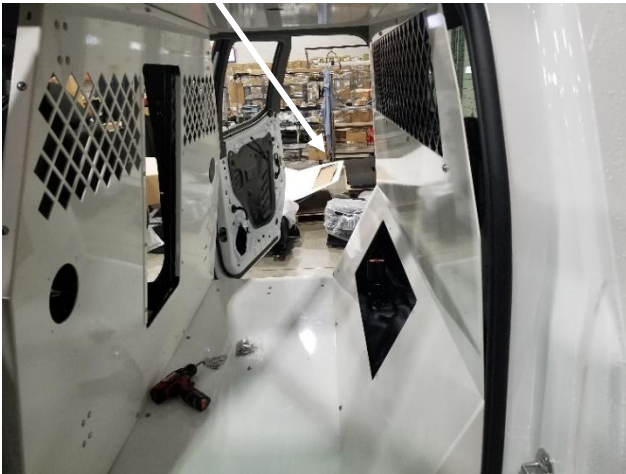
Loosely install bulkheads, rear support, and roof panel using the 1/4" Phillip screw, 1/4" Flat washer, 1/4" x 3/4" Carriage bolt and 1/4" Serrated nut.
