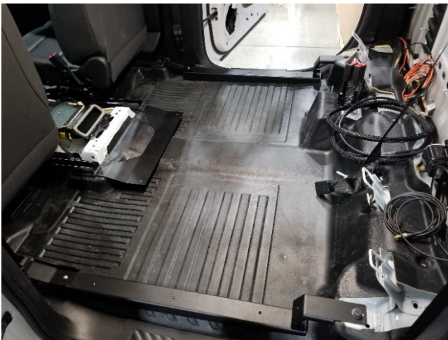
Assembled floor bracketry should look as shown. Some hardware in photos has changed for production.
