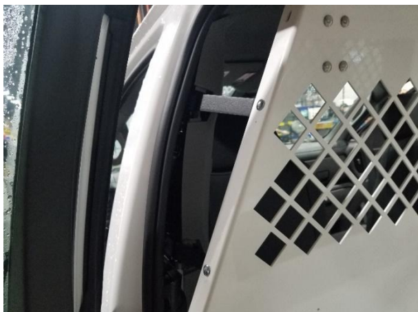
If installing side drawer storage see last page. Tighten remaining loose bulkhead and bracket hardware.
