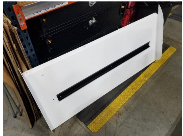
Attach floor stiffener to floor panel with 1/4" Phillips screw and 1/4" flat washer.
