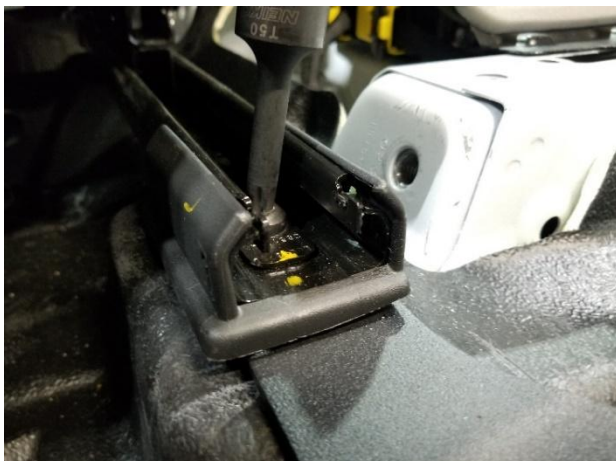
Install floor panel, align to be centered and square, and tighten all hardware.
