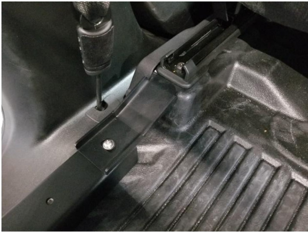
Place supports on floor. Slide front brackets under seat tracks and loosely install 1/4" Phillips screw and 1/4" Flat washer.
