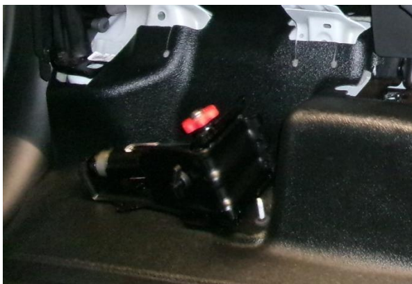
Remove the jack and relocate where appropriate.
