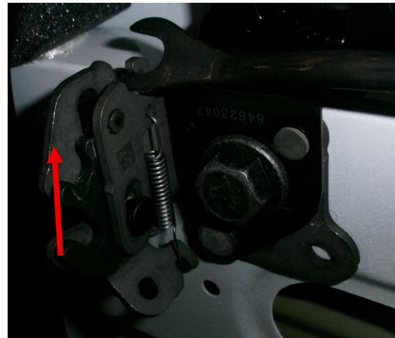
Push up the rear seat back latch to remove the seats. Remove the middle latch.
