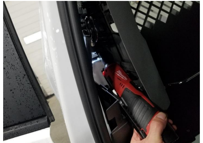
Attach B-pillar brackets and tighten hardware. Reinstall trim once tight.
