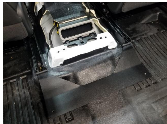
Remove rearmost bolts of front seat tracks and the center seat or console. Slide tunnel bracket under seat tracks and loosely reinstall hardware.
