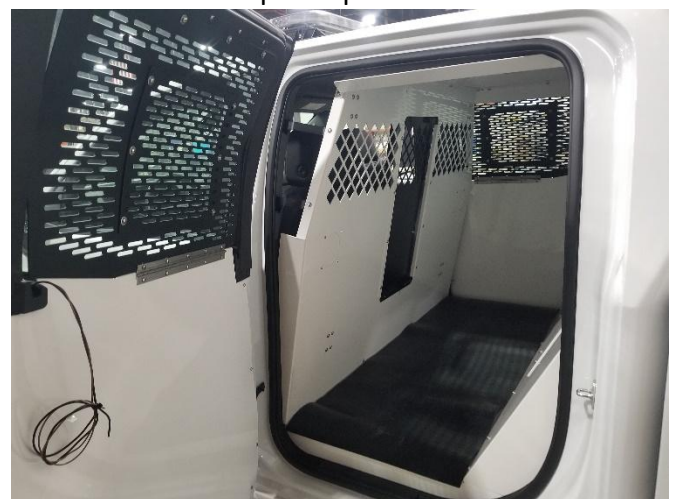
Install door panels and window guards, insert floor mat, install rear cover panel and window using #10 x 1/2" Screw and #10 x 1/2" Flat head screw. Install any optional accessories at this time.
