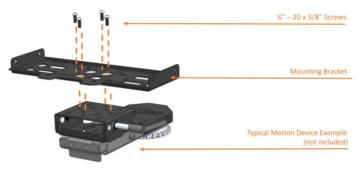
NOTE: We recommend applying a drop of medium strength (blue) thread locking adhesive to the threads of all fasteners.
