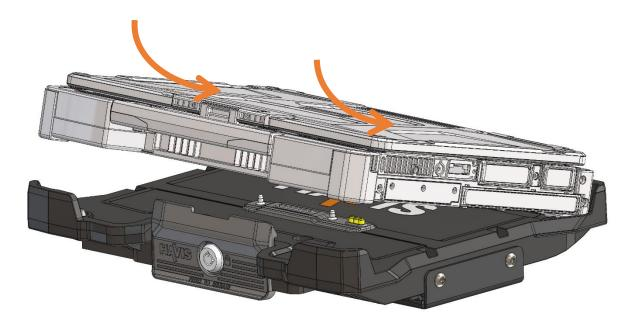
4) Lower front of computer onto Docking Station, ensuring computer properly aligns with the front fence on the Docking Station. Apply downward pressure to the front of computer, until Front Hooks on Docking Station snap into place and secure the computer. Ensure Front Hooks are fully engaged by trying to pull up on the laptops handle.
