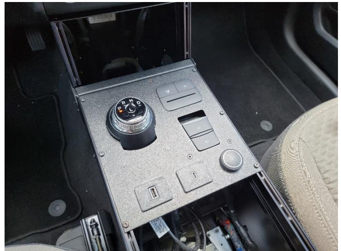
Install shifter plate on console using (6) T-20 Torx head screws.
