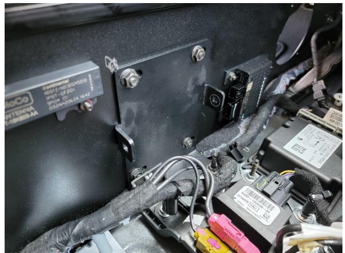
Attach to mid-mounting brackets to housing with 1/4" x 3/4" carriage bolts.
