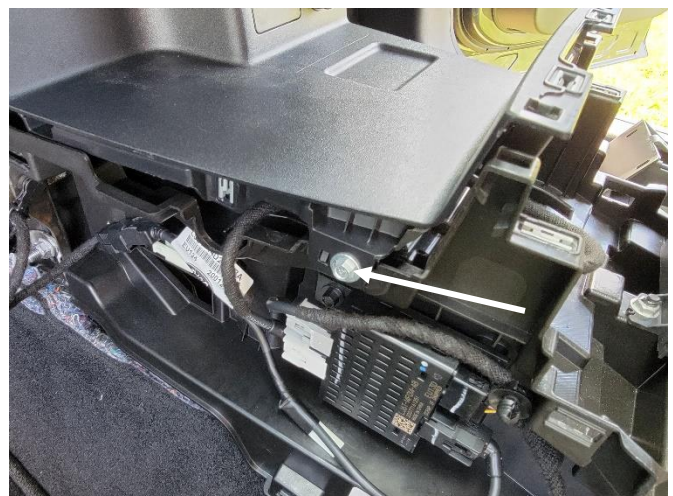
Remove 10mm head fastener from center, USB plate.
