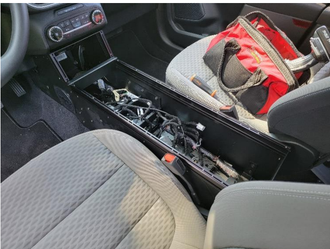
Place console in vehicle. Slide up to dash.
