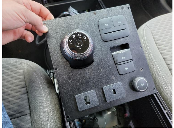
Verify all modules are attached, snug and no buttons are binding.
