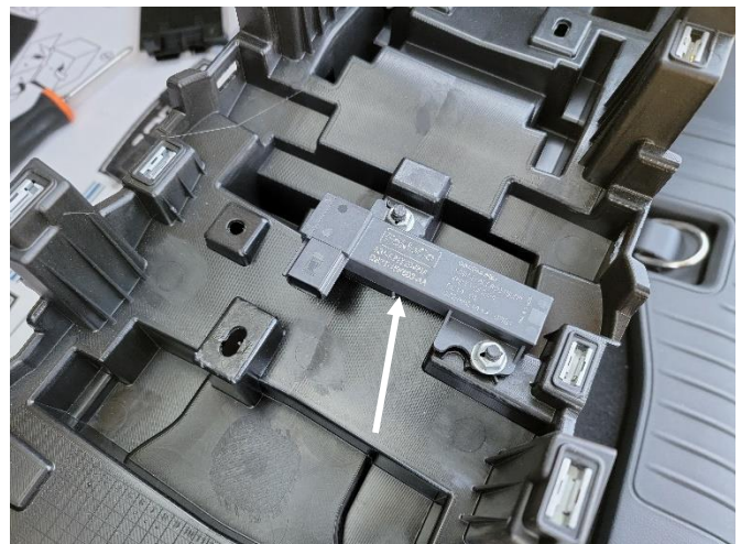
Remove secondary key sense module from top of OEM console.
