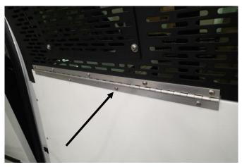
Align the hinge mounting holes to holes in the Havis DP-C26-A door panel. Attach hinge with # 10 x 1/2 Phillips pan head sheet metal screws. OEM door panel will require 1/8" pilot holes for attaching hinge with same screws.
