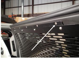
Mark and drill 5/32" holes in door / window frame for upper bracket. Screw upper bracket to door frame with # 10 x 1/2" flat head sheet metal screws.
