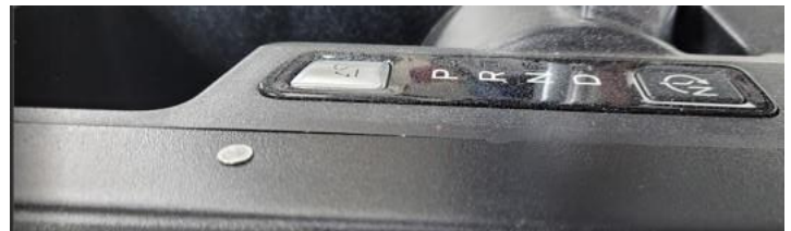
Tighten the three 1/4-20 Nylock nuts and 1" fender washers until the shifter sits flush with the center console bracket.
