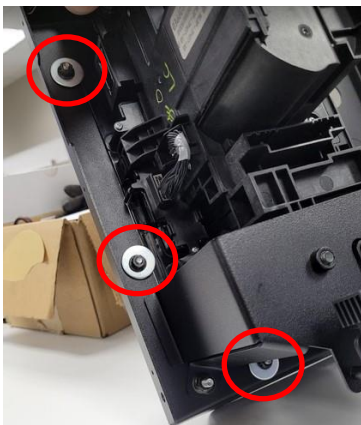
Loosely attach three 1/4-20 Nylock nuts and 1" fender washers to threaded studs near shifter. Note: Washers should seat underneath shifter lip.
