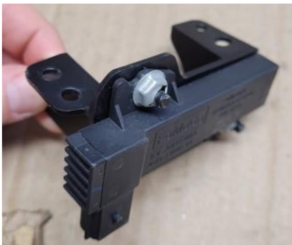
Remove keyless entry antenna with its mount from underneath the cup holder. Remove the antenna's mounting screws. Do not remove the captive nuts.
