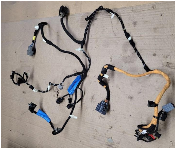
Remove wiring harness from OEM console. Note: OEM console lighting does not need to be removed because it will not be used.
