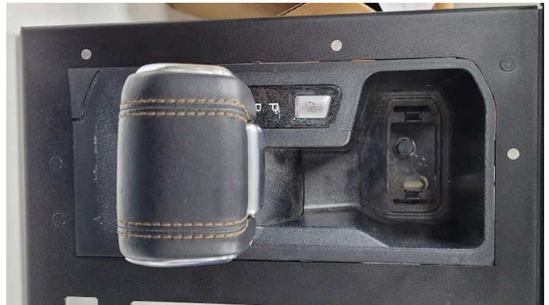
Center shifter in cutout and tighten all hardware. Note: Tighten 5/16-18 screws before tightening 1/4-20 nuts.
