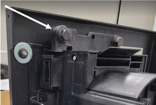
Loosely attach shifter to rear mounting bracket using 5/16-18 X 1-1/4 bolts, split lock washers, and washers.
