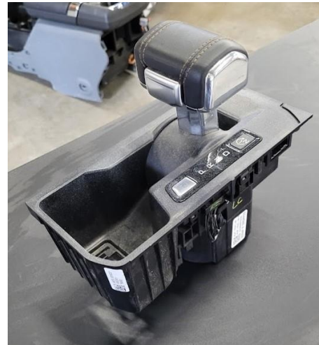
Remove shifter, all charging port modules and power plugs from OEM console.
