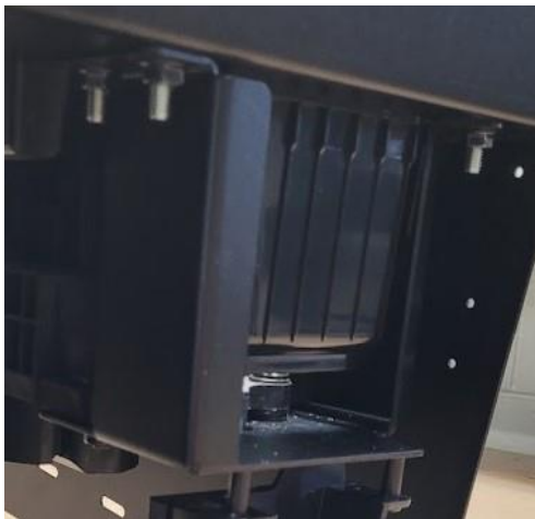
Loosely attach shifter to front mounting bracket using 5/16-18 X 1-1/4 bolts, split lock washers, and washers.
