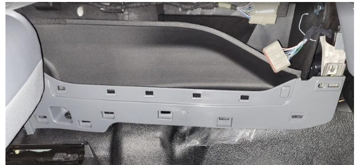
Remove OEM console by detaching side trim panels, disconnecting wire harness and removing six mounting screws.
