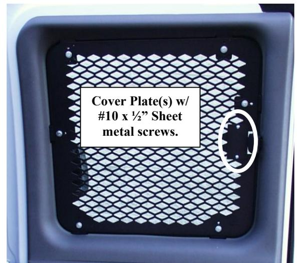
The WGI-C1-2X (21160) extension plate will be located behind the OEM AC ductwork and attaches to the rear side window guard WGI-C1-2 (21159) or WGI-C3-2 (21190) and window frame with hardware and brackets provided.
