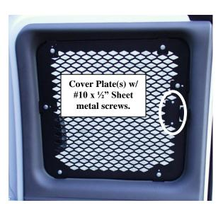
The WGI-C1-2X extension plate will be located behind the OEM AC ductwork and attaches to the rear side window guard C-WGI-C1-2 or WGI-C3-2 and window frame with hardware and brackets provided.
