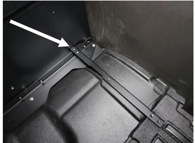
Position DS and PS Front Floor Brackets on the lower flange of the K9-C26-XL/PT rear bulkhead as shown.
