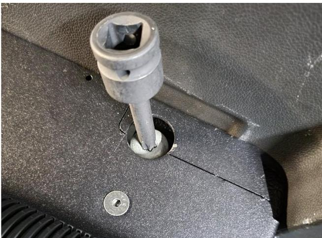
Loosely attach rear floor brackets to rear seat belt anchors on each side with OEM 12mm Torx bolts. Add 1" hole plug after hardware it tightened.
