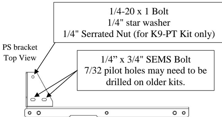
Attach the PS and DS floor brackets using supplied 1/4" hardware.
