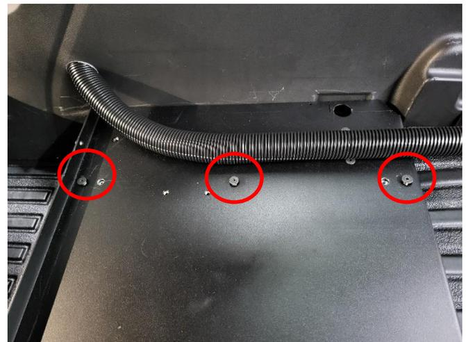
Loosely attach base plate to front floor brackets using supplied 1/4" x 1/2" Flat head bolts. (3 each side)
