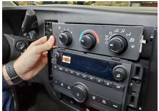
Re-install HVAC controller using 8-32 x 1/2" screw and #8 star washer.
