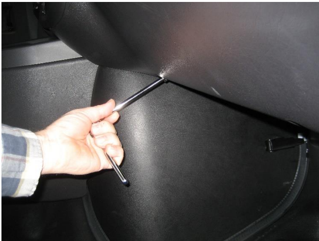
Carefully remove passenger side lower dash panel. It may not be necessary to be completely removed. (10 mm socket)
