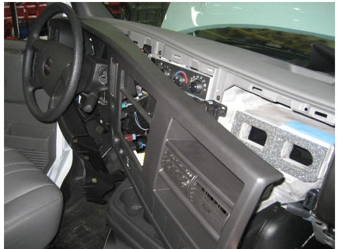
Detach center dash panel and pull out passenger side only as far as needed to remove the AM/FM
