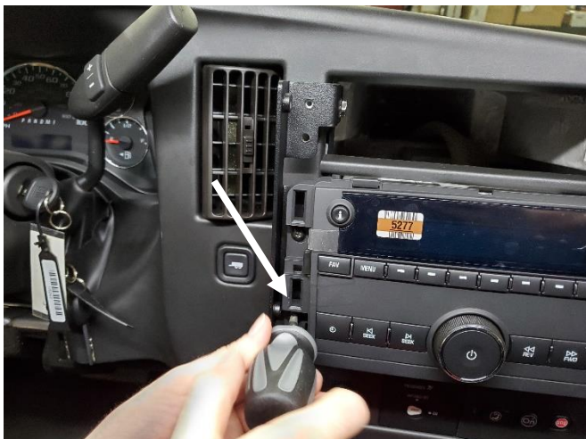
Attach using 8-32 x 1/2" screws and #8 star washers.
