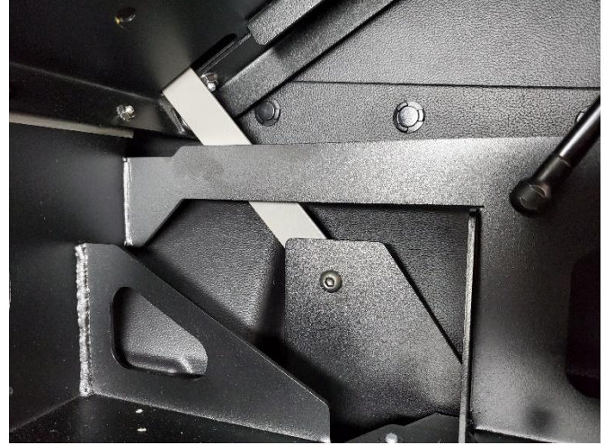
Attach to PROKIT-2 bracket using hardware supplied with Pro-Gard partition.
