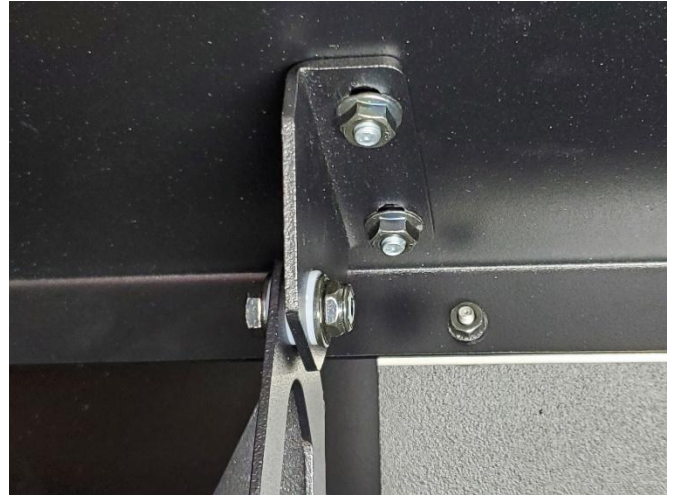
Mounting tabs for TTP-4 are slotted; adjust as needed to ensure smooth latching and unlatching of tray.
