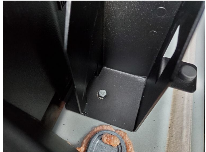
Loosely attach rear latch pedestal to OEM threaded holes in floor using M6 bolts and 1/4" washers.
