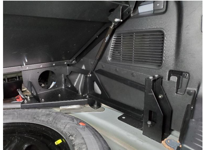
Attach gas springs to ball mounts. Be sure to have body of spring at the top.
