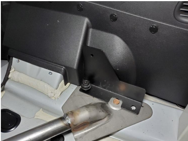
If using a Pro-Gard rear partition, optional PROKIT-2 is required. Remove the rear mounting bolts for the crash brace. Place the PROKIT-2 brackets on top of the crash brace and loosely install the forward bolt.
