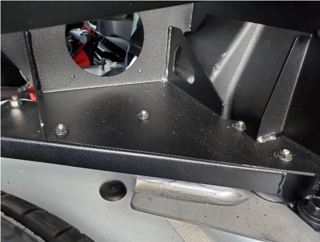
Attach to "X" brace mounting bracket studs using 1/4" serrated nuts. Once both sides are lined up, tighten OEM hardware and U-bolt
