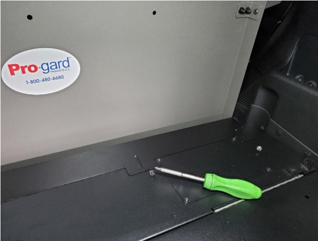
Attach forward trim panel and electronics access covers to top of 1201 using (4) 10-32 x 1/2" screws and washers. Slide trim against partition and tighten hardware.
