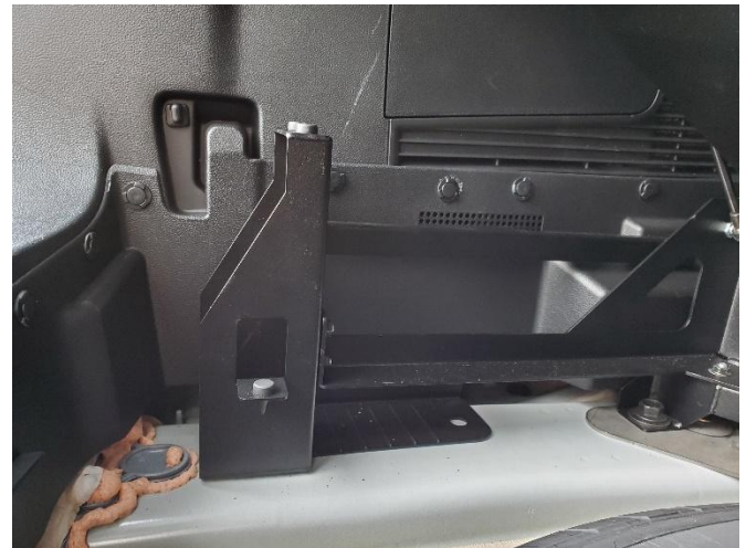
Line up lower mounting support arm to rear pedestal mount studs and attach with 1/4" serrated nuts.
