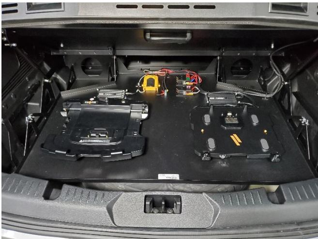
Example of C-TTP-INUT-4 with equipment mounted.
