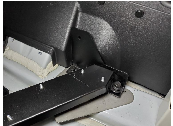
Place the TTP mounting bracket over the PROKIT-2 mounting bracket and install the rear OEM bolt. (Do not tighten hardware yet)
