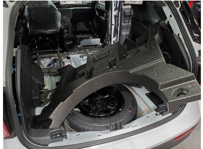
Remove OEM foam sections from rear of vehicle. (These will not be reused)
