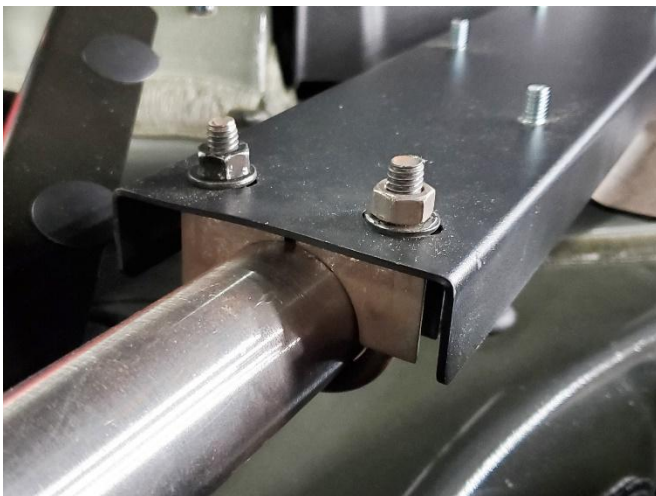
Attach other end of lower "X" brace bracket with supplied U-bolt, flat washers, lock washers and nuts. Repeat for other side
