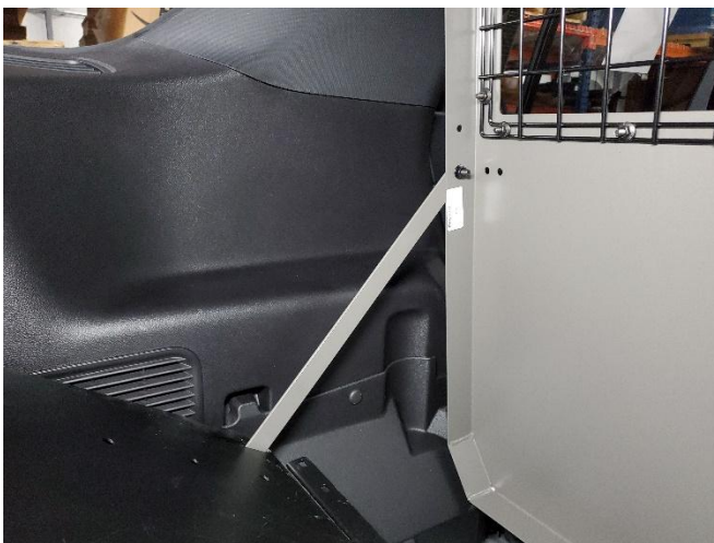
If using PROKIT-2 along with a Pro-Gard rear partition, install the rear support braces through opening in top of TTP. Older TTP trays may not have the slots for the support arm. Slots will have to be cut in these instances.
