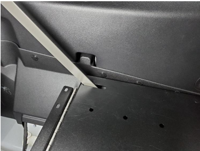
If using PROKIT-2 along with a Pro-Gard rear partition, install the rear support braces through opening in top of TTP. Older TTP trays may not have the slots for the support arm. Slots will have to be cut in these instances.
