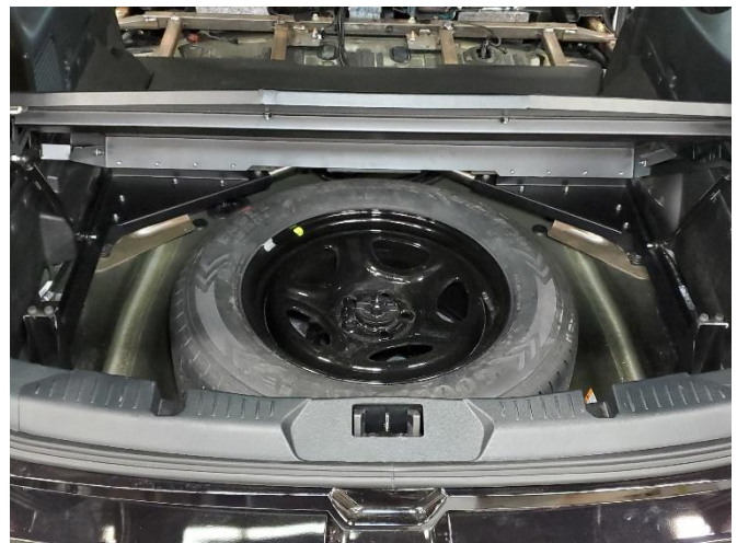
Carefully place top mounting platform into rear of vehicle and onto the lower mounting brackets.
