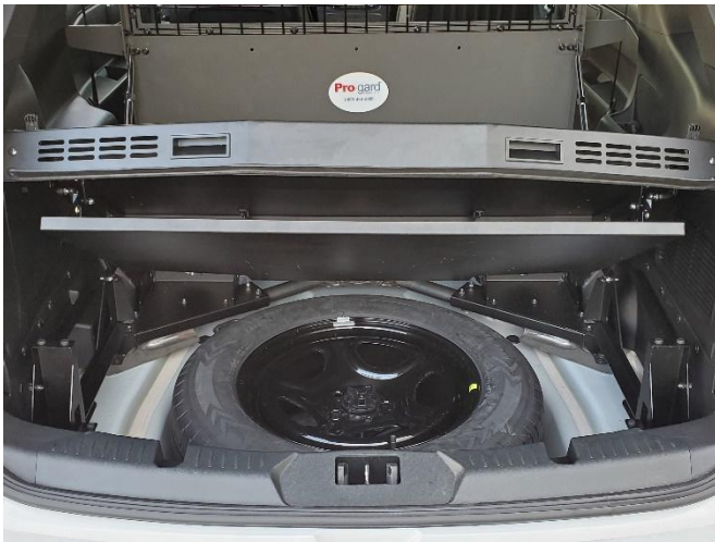
Open and close top platform and lower tray to confirm proper function.
