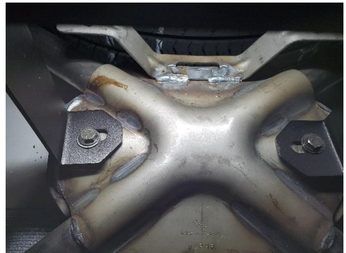
Attach CM010302 front support legs to OEM "X" brace using (2) 3/8" x 1" bolts, washers, and nylock nuts.
