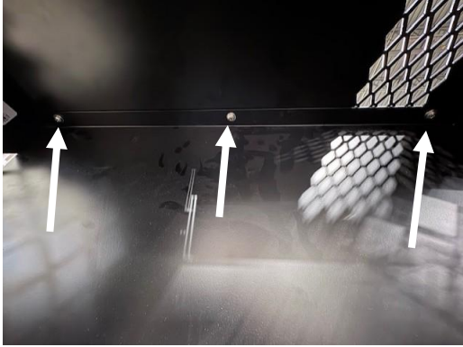
Loosely attach divider (55285/55286) to ceiling using three (3) 1/4" x 3/4" Phillips pan head machine bolts and flat washers.
