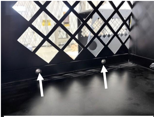
Loosely attach top shelf to rear bulkhead/rear window screen using two (2) 1/4" x 1/2" carriage bolts and serrated nuts.
