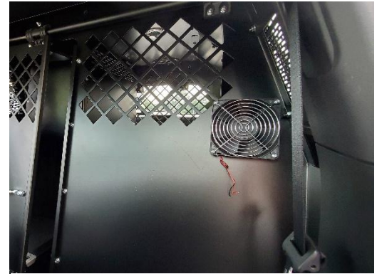
Example mounting location for the optional air circulation fan.
