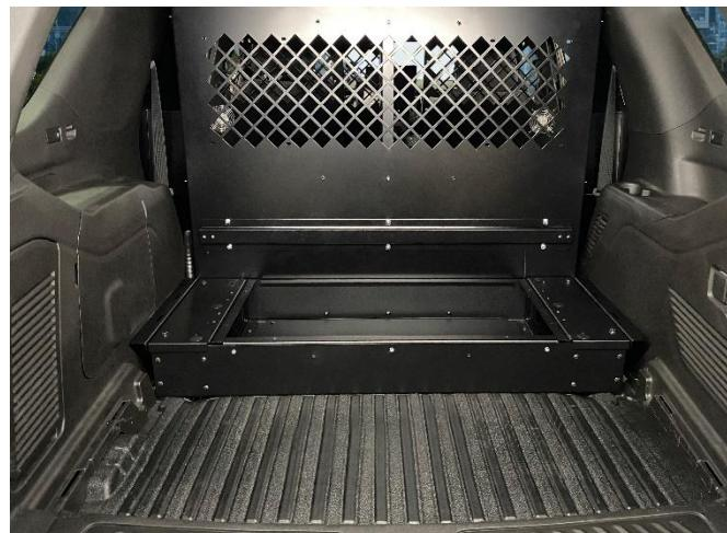
Place main box assembly onto brackets and attach with (10) 1/4" x 3/4" Hex bolts and star washers.
