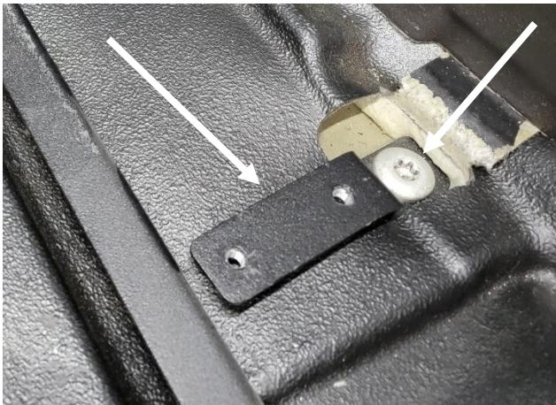
Locate OEM rear floor seat belt anchor bolts.
