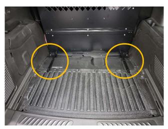
With K9-C26-XL or –PT installed, place driver and passenger side front floor brackets into vehicle.
