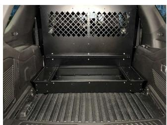
Place main box assembly onto brackets and attach with (10) 1/4" x 3/4" Hex bolts and star washers. Mount equipment onto removable tray as desired.
