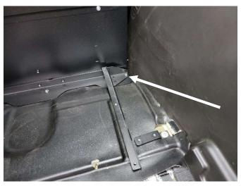
Attach each front floor bracket to 1/4 x 3/4 bolts in K9 rear closeout bracket. Also attach to pre-drilled holes with two (2) 1/4 x 3/4 self-threading screws. For K9-PT model, attach passenger side bracket with one (1) 1/4" x 3/4" Hex bolt and serrated nut.
