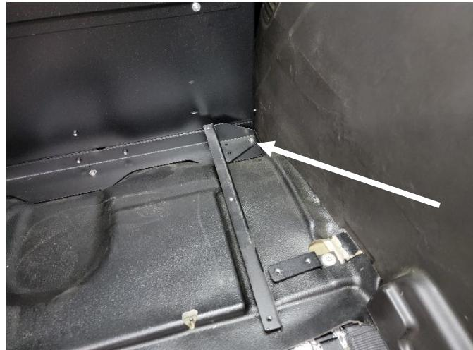
Attach each front floor bracket to 1/4 x 3/4 bolts in K9 rear closeout bracket. Also attach to pre-drilled holes with two (2) 1/4 x 3/4 self-threading screws. **For K9-PT model, attach passenger side bracket with one (1) 1 1/4" x 3/4" Hex bolt and serrated nut.**
