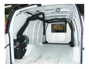
Route HVAC 2 1/2" blower hoses to the approximate locations with tape along ceiling where they will be installed into the ceiling after insert is installed. Mount hoses with wire ties at wall and ceiling corners only. Leave enough slack to reach hoses for permanent mounting.
