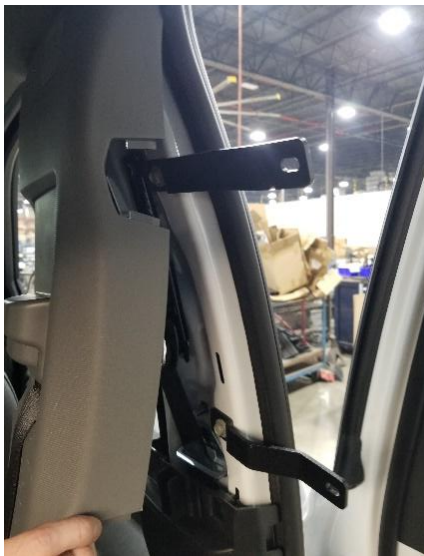
Replace grab handles with B-pillar brackets, leaving trim loose.
