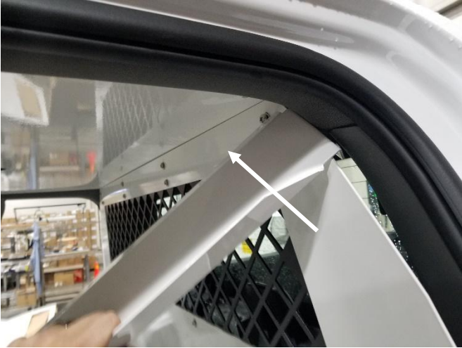
Hook top of side curtain panels over bulkhead and rotate up into place to install.
