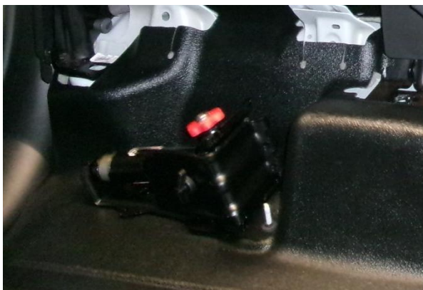
Remove the jack and relocate where appropriate.
