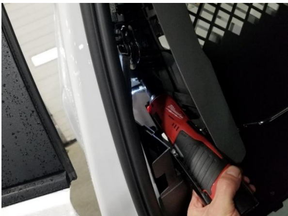
Attach B-pillar brackets and tighten hardware. Reinstall trim once tight.
