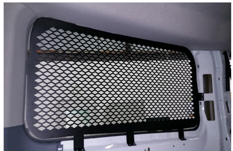
Hang the screen with only a few screws and then mark and drill the remaining mounting holes.
