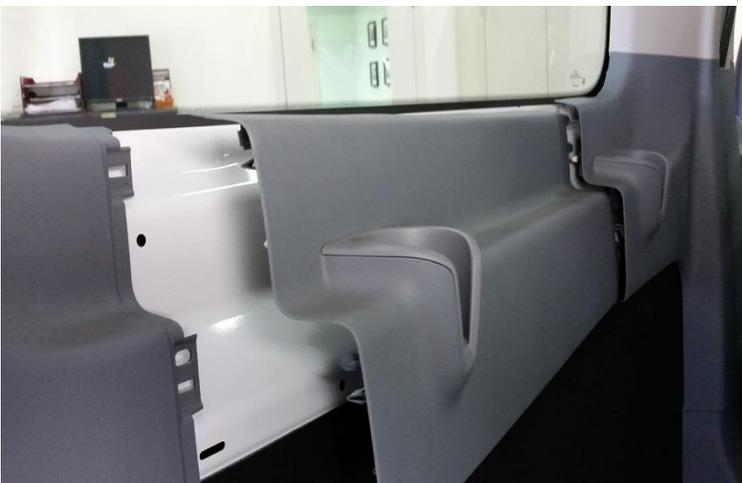
Carefully remove the vans interior panels including the door panels.
