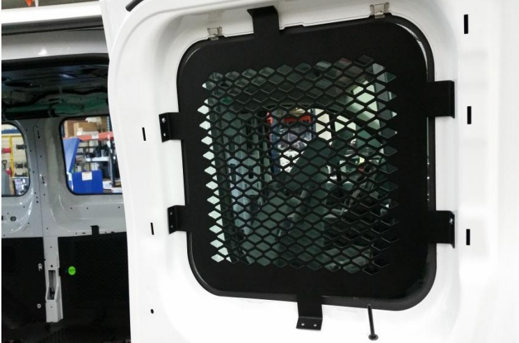
Determine location of each guard. Place guard up to the window frame, mark and pre drill mount holes with a 1/8" drill bit. (Slight bending of the tabs may be necessary to ensure a proper fit)
