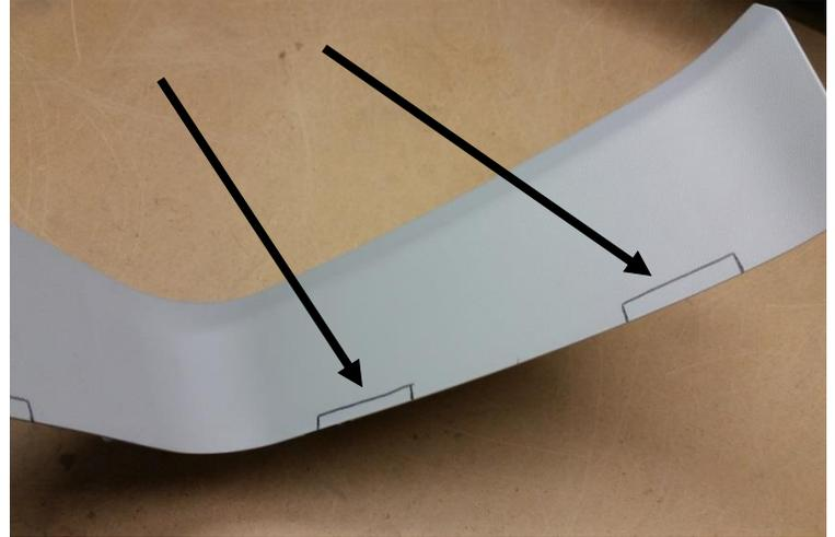
When all guards are hung, begin to loosely place the trim panels back on the van. Mark the trim on either side of the mounting tabs for notching.
