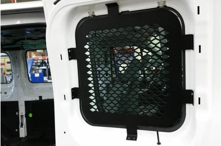
Determine location of each guard. Place guard up to the window frame, mark and pre drill mount holes with a 1/8" drill bit.
