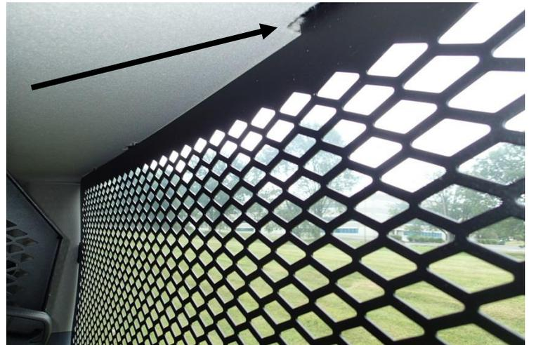
When reinstalling the trim, additional notching may be necessary. Cut as needed.
