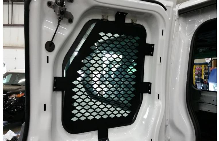
Attach screen to door using #10 x 1/2" screws
