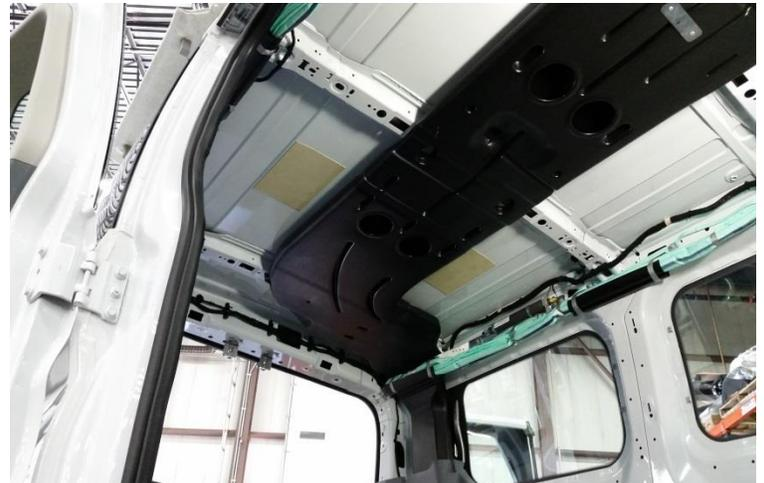
Removing the headliner is recommended but not required. Removing the headliner will be required if installing a Middle Partition. If installing a middle partition it is recommended to mount the upper brackets now. Refer to the P-MID-3 instructions for proper bracket placement.
