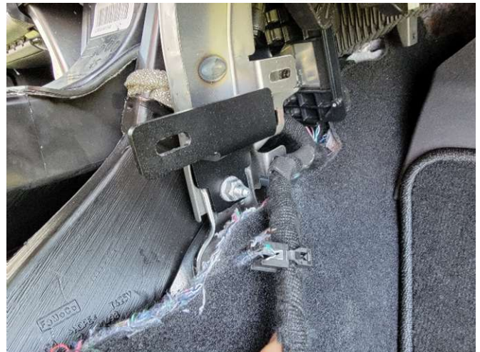
Install Passenger side forward mounting bracket.
