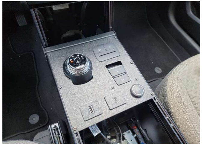
Install shifter plate on console using (6) T-20 Torx head screws.
