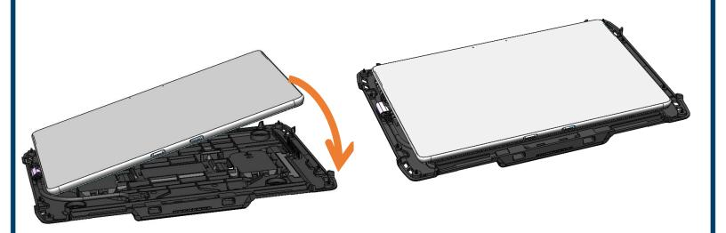
4) Place the Front Assembly of the Tablet Case on the Back Assembly. Ensure a proper fit by looking for gaps along the seam between the two pieces. This case contains six snap fits denoted with the arrows below. Apply light pressure around the entire perimeter to ensure that all six snaps engage.
