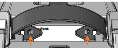
2) With the front cover removed. Insert the USB connector from the Back Assembly of the Tablet Case into the circled USB port of the tablet (*TC-401 shown as example*).
