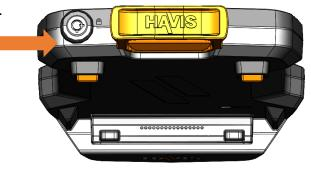
2) Hold Tablet in landscape orientation, with bottom angled toward Docking Station. Lower Tablet onto the Docking Station so the Alignment Pockets on the Tablet Case align with the Front Hooks on the Docking Station.
