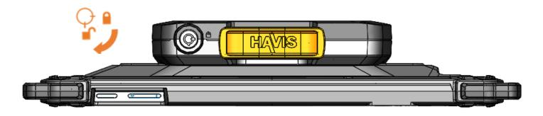
2) While holding Tablet Case with one hand, lift the Release Handle on the top of Docking Station.
