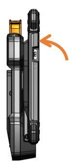
4) For theft deterrence, secure Tablet Case by locking Docking Station with supplied key (Hardware Kit Item 2).
