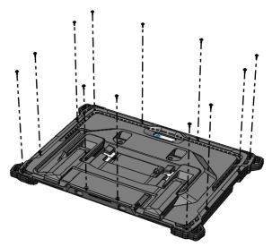
6) To remove your tablet from the Tablet Case remove all the screws then carefully turn the case over. If your Tablet Case includes interlocking snaps use your fingers to pry the Front Assembly up from the inside edge along the screen. Lift the Front Assembly off the Back Assembly, unplug the connector, and remove tablet.
