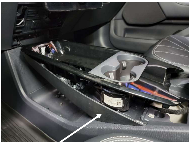
Unsnap and remove top of center storage area.
