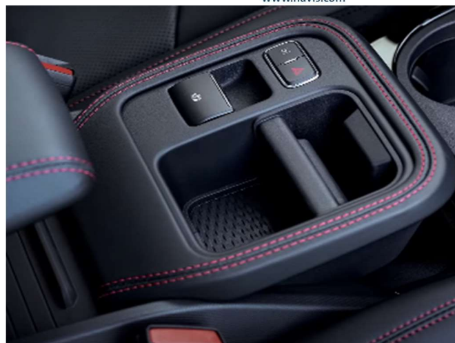
Remove front OEM console by gently pulling up from the front.
