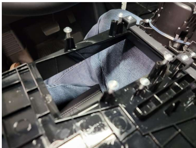
Unscrew wireless phone charger from underside of center storage area.
