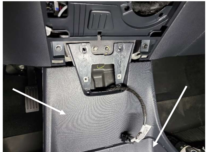
Remove forward panel and lower center storage area.
