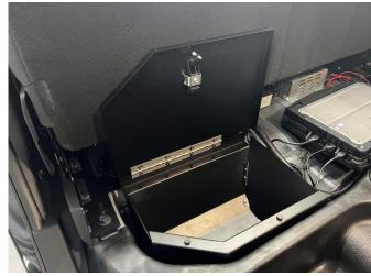
Place SBX box(es) into appropriate location, line up 2 mounting points with front seat bolt and use Hex M12 x 1.75 x 35 with washer for the rear, install two 7/16 ¾ lag bolts on the front edge towards the front of the vehicle
