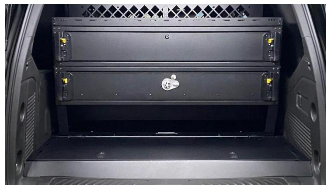
Attach main box lid with  $1/4''$  x  $5/8''$  Button head screws. Attach risers to main box with  $5/16''$  Hex bolts and washers. Attach risers to drawer with  $5/16''$  Thread-Forming Screws.
