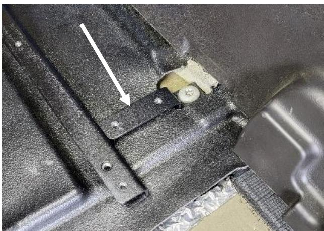
Loosely attach rear floor brackets to rear seat belt anchors on each side with previously removed OEM 12mm Torx bolts.
