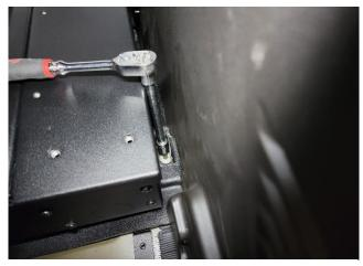
Tighten floor bracket hardware.
