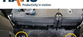
Determine 3rd row seat bolt locations in forward floor and loosely attach long front brackets with supplied M10 bolts.
