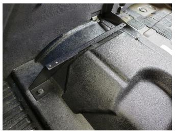
Passe ager side bracket shown attached to floor with M10 x 1.5 x 45mm hex bolt.
