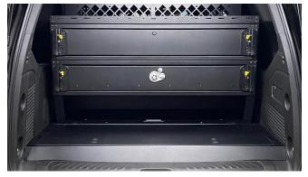
Attach main box lid with 1/4" x 5/8" Button head screws.
