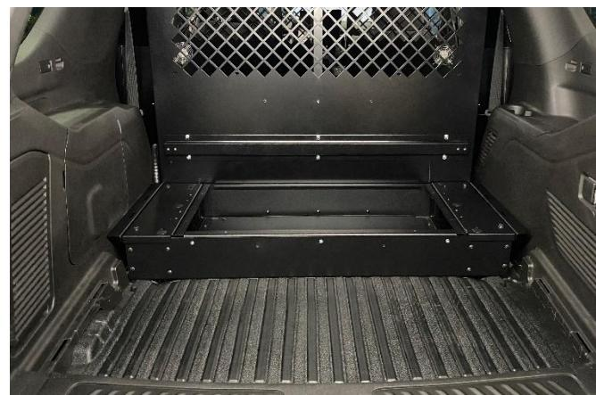
Place main box assembly onto brackets and attach with (10)  $1/4''$  x  $3/4''$  Hex bolts and star washers. Mount equipment onto removable tray as desired.
